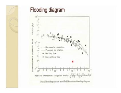
Now, because we would certainly do not want to operate the blast furnace above the flooding limit; otherwise the efficiency will degree the blast furnace will hang the operation will hang and then one had to set it down. So, lots of work has been done and this is similar to many chemical reactors, they also do not operate above the flooding point.
