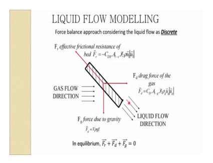
So, essentially you have three resistance; the effective frictional resistance of by the packing that is what you called the bed resistance, then you have the gate drag force, which is acting on the liquid.
