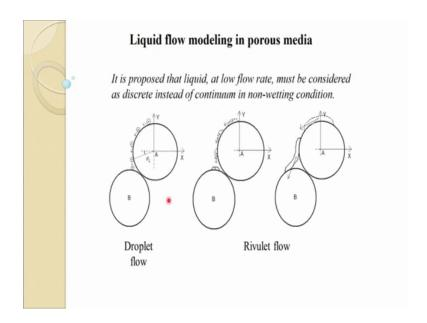
So, another theory has been proposed for this; so it is proposed that liquid, at low flow rate, must be considered as discrete instead of continuum in non-wetting condition. So, we said about the discrete liquid flow. So, when we said discrete, which means this like in a not a continuous way, it is in breaking form.
