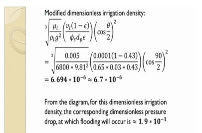
So, what we have to do? We have to first calculate this x axis. So, irrigation density, which is given by this; so viscosity is 0.005 Pascal second from our previous example, density of the liquid 6800 kg per meter cube, and the gravitational constant 9.81, then you have the velocity of the liquid 0.0001 meter per second.
