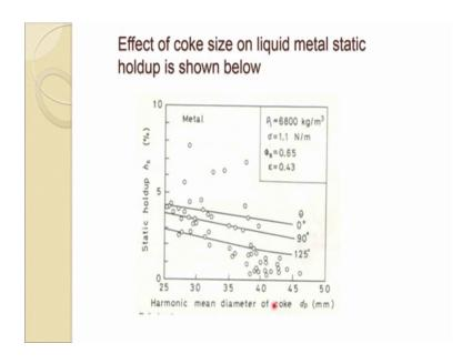
So, efficiency of the reactor does not affect. This figure shows the effect of coke size on liquid metal static holdup. So, you can see this is actually let me tell you, the actual live blast furnace result when I say the live which means the blast furnace has been quenched and dissected and then the data were collected. So, it is in the actual blast furnace.
