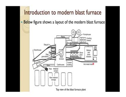
So, this below figures shows a layout of the modern blast furnace, it is a top view. So, this is showing about the raw material from where the iron ore, coke, flux, sinter or pellet whatever it goes to there and using the conveyor belt drops into the blast furnace. Then you have a slag granulations unit slag pit stock house, then you have a gas cleaning unit and juban the gas and the stove and you put it through the tuyere, the hot airs and hot metal track is over there.
