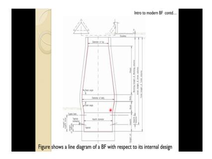
And this gives a line diagram of the internal design of the blast furnace. So, you can see for the throat region the diameter, and all this even this strake stake region and bosh region they have a particular angle like a stake angle and bosh angle and these are very important, depending on the quality of the raw material their (Refer Time: 05:00) angle and others. So, for a smooth flow of the solid these are very important.
