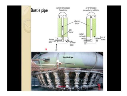
The bustle pipe this is actually if you look at that gas is injected gas and fuel other they can injected through the tuyere and this is very important person and that one. The point is this because they are about 30, 40 tuyeres around the circumference of the blast furnace, and it is necessary that all the tuyeres should have the right pressure and should deliver the right amount of the gas or fume.
