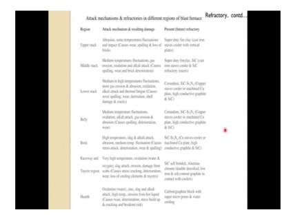
And this slide. In fact, gives you or shows you about the attack mechanism and the refracted which one should use.
