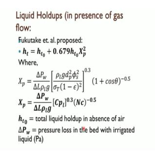
And in presence of gas flow they proposed this correlation, where h t is the total liquid holdup; which is nothing a combination of static and dynamic holdup, but in presence of gas flow, ht naught is again the total holdup, but in absence of gas flow. So, this is a total a holdup in absence of gas flow this is a total holdup in presence of gas flow.
