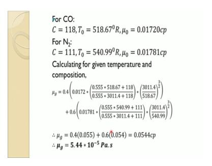
And once we substitute into this equation so for CO: C equal to 118, T naught in (Refer Time: 24:44) similarly for nitrogen is 0.111 one what the (Refer Time: 24:49), then the mu naught viscosity at a temperature is given, so we then we can calculate for the given temperature, what would be the this viscosity.
