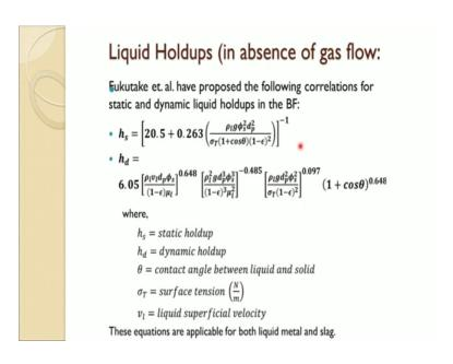
So it is quite difficult to quantify this liquid holdup especially at this high temperature. So, people have done the experiment again in the cold condition the way that now we saw in; this previous video. In the same way people have done the; experiment to quantify liquid holdup, static and dynamic using the room temperature experiment.
