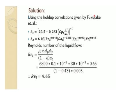
So, using that holdup correlation, so what we have to do; we have to calculate Reynolds number, Galileo number, Capillary number, interfacial force. So, Reynolds number and packed way is given by this shape factor. So, density is given superficial velocity is given 0.1, particle size is given 30.
