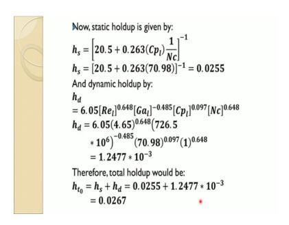
So, once you now all these non dimensional quantity, now you can substitute them into the correlation static holdup you put that, so you get about 0.0255 meter cube per meter cube. Remember this unit with respect to the packing volume and dynamic holdup you get 1.2 into 10 to the power of minus 3. So, if you look at this, you can see the dynamic holdup once is usually in these conditions in the blast furnace; they are one order magnitude lower than you are a static holdup of the liquid.
