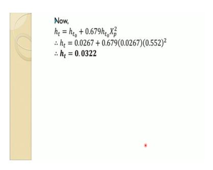
And now this Xp we can put in the total liquid holdup equation which is nothing as we have seen the total liquid holdup in presence of air is equal to total liquid holdup in absence of air plus this term. Now, Xp we have calculated total holdup in absence of gas, we already know from previous example. So, once we put these quantities all together we get the total holdup 0.0322.
