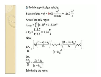
Now, the average diameter of the belly and blast region is given, which is about 12 meter. So, using that, we can get the area of the belly region. So, that comes around 113 meter a square.
