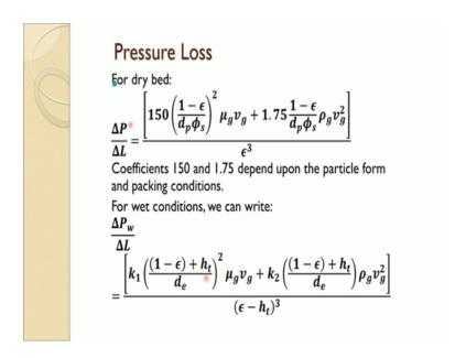
So, naturally one has to know then this; and for dry bed you already know about it, using the argon equation we have used this one many of the application previously, so for dry bed you can calculate the pressure drop per unit length using this argon equation, where coefficient are used 150 and this and this coefficient it is a depends on particle form and the packing condition.
