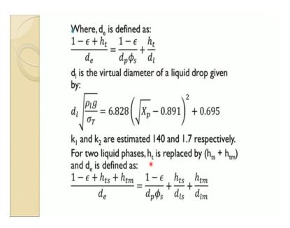
So, these define this way and, where dl actually is the virtual diameter of a liquid drop given by this formula. So, you can easily once you know that these properties are known to you can calculate it.
