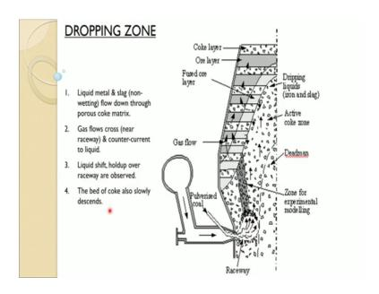
Ok, now we will start talking about a dropping zone, which is very important zone in the blast furnace. This dictate all the aerodynamics of the blast furnace vocalized-noise] and figure shows the dropping zone which you are already familiar by now.
