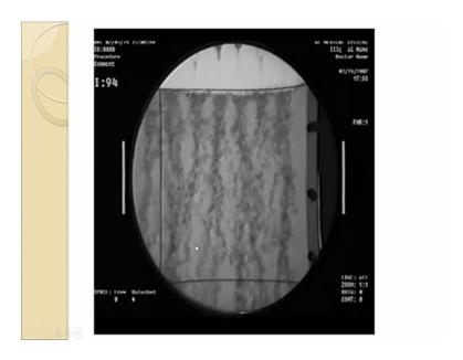
So, you can see that this is a dry bed in the starting and then liquid from the top is a fall through the trips.
