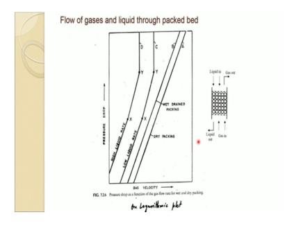
So, it is a quite complex process and we will be talking a little bit more on that. So, if we take a flow of gases and liquid through packed bed this figure represent what happens. So, when gas is flowing upward liquid is flowing downward the situation is known as counter current system which you are already aware of it from our last lectures.
