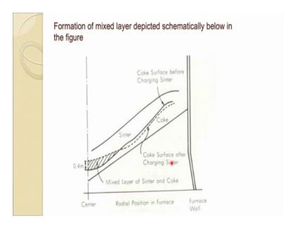
So, in formation of mixed layer; so, when actually you are charging the material say on the top of the coke layers you are charging the sinter. So, at naturally at the impact point, this coke will displace which you have seen in the previous one. And during the charging of the sinter and coke is at the bottom you will see previous profile of the coke layer was this after charging the sinter it became like this.
