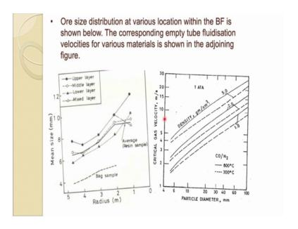
This figure shows the size distribution at various locations within the blast furnace and corresponding empty tube fluidization velocity for various material.
