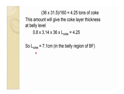
And now again you can calculate the volume of that and equate with this tons of coke you can get the value of the coke layer thickness in the belly region which comes about 7.1 centimetre thickness in the belly region of the blast furnace. So, that is keeps you some idea how you can calculate that on the reaction and other parameter which is given the layer of the material in different different region and you can try to maintain it.
