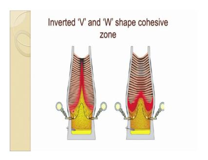
So, I like a messy zone what we call it. So, this brown one is becoming fluid. So, when it becomes fluid which means the gas cannot flow through that, already ore has a very low void fraction. So, gas already feels quite a big resistance and now in this condition where it has fluid the gas cannot flow through that.
