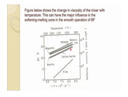
This figure shows the change in viscosity of the mixture with temperature and this can have a major influence in the softening melting zone in the smooth operation. So, as we said the gas flow is very important.
