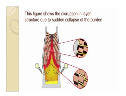
The next figure you will see what may happen. Due to the slipping the layer is texture get disturbed, and once the layer structure get disturbed you have a very big problem with the gas flow. Gas is feeling more resistance like in this one the layer structure as gone this now case has to troubled not only the longer part even the resistance it has though fetch through that.
