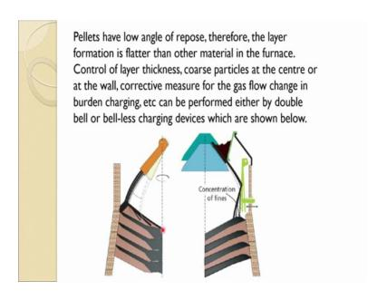
So, pellet us have low angle of repose therefore, the layer formation is flatter than other material in the furnace. Control of layer thickness, coarse particle at the centre or at the wall corrective measure of the gas flow change in burden charging etcetera can be performed either by double bell or bell less charging devices which are shown below.
