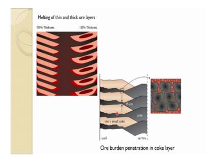
So, this shows about the ore layer thickness. So, normal 100 percent thick and if you are increasing the thickness, essentially what is happening at the centre of it is not getting reduced properly and this travels down. And then this reduction will occur in the lower part of the furnace where the director reduction and then more heat would be consumed endothermic and as we discussed the chilling and other effect can come into the picture and operation may not be a smooth one.
