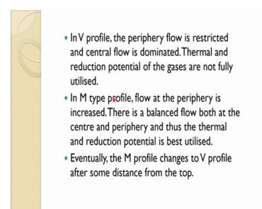
So, in V profile, the periphery flow is restricted and central flow is dominated. Thermal and reduction potential of the gases are not fully utilized. In M type profile, flow at the periphery is increased. There is a balanced flow both at the centre and the periphery and thus the thermal and reduction potential is best utilized.
