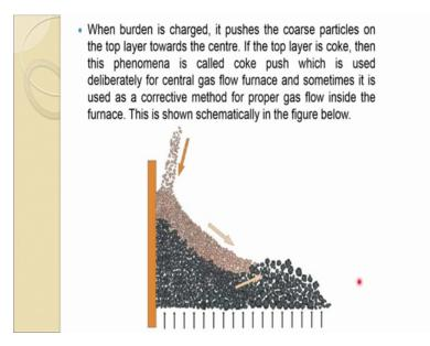
So, we will see, so when usually when burden is charged you can see in this 1 this is more about the pushing of the coke, but mostly you will look at the profile of this will go bit like this while profile of the coke would be much sharper. So, when burden is charged precise the coarse particle on the top layer toward the centre if the top layer.
