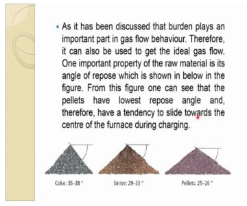
Now, another important property of the raw material is about the angle of repose. So, it has been burden plays an important part in gas flow behaviour as we have seen in the previous slides therefore, can also be used to get the ideal gas flow.
