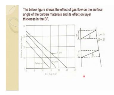
This next figure; showing the effect on the surface angle the effect of gas flow on the surface angle of the material. So, as you can see that when the gas flow increases of course, in rho u square term essentially the your surface angle decreases for coke sinter
