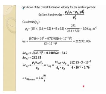
So, for the fluidization as you know the first you have to find out the Galileo number and that we have to take now it is asking about the critical minimum critical velocity. So, minimum critical velocity has to be related to the minimum particle size diameter.
