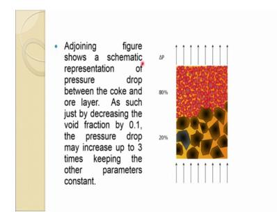
So, this figure shows about the schematic of an ore particle and this is the coke as you can see from the previous event slide that the size is almost 3 to 4 times different than the coke size. So, essentially one would expect a very high pressure drop in this smaller size particle then the larger 1. So, the black one is representing more as coke and this one more as iron bearing material sinter or pellets or even the ore.
