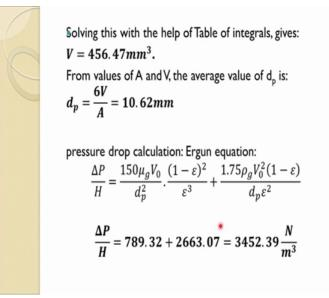
Then, so in this when you have to use table of integrals this and as you can get the volume about 456 56 millimetre cube. So, from this value now we can calculate average diameter of the particle which comes 10.6 millimetre.
