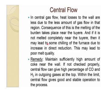
Now, how to so in central gas flow heat losses to the wall are less. Due to the less amount of gas flow in that region consequence of this is the melting of the burden takes place near the tuyere.
