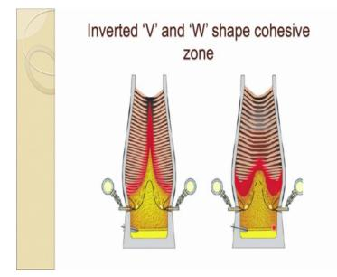
And this is a w shape cohesive zone. So, you put the more coarser material in this case at the centre, centre. So, central gas flow is there. So, gas can easily pass through this region; however, in this case as you put more coarser particle toward the periphery, and less over here.
