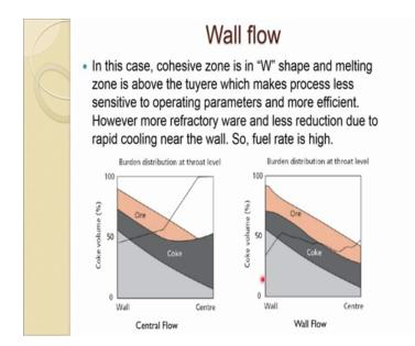
So, another in the wall flow what is happen in this case cohesive zone is in W shape, and the melting zone is above the tuyere which make process less sensitive to operating parameter and more efficient; however, more refractory ware it is a more refractory ware and less reduction due to the rapid cooling near the wall, so fuel rate is high.
