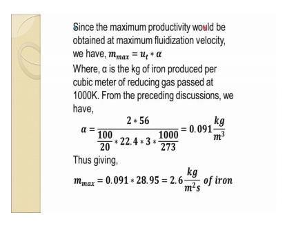
So, 3 moles. So, again now utilization factor for this reducing gas is only 20 percent. So, this you multiply it with that, then this is the volume which out the gas which you need to produce 112 kg iron and since the maximum productivity also is related with the
