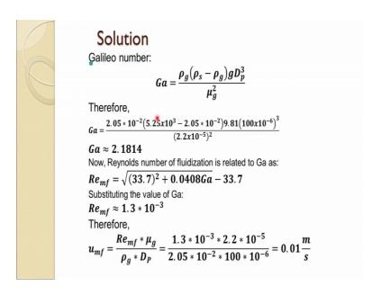
So, particle size also makes a big difference in the minimum fluidization velocity. So, this is the second part of the question which be answered and the third one is about that filtration velocity and this is once we know minimum fluidization velocity in elutriation velocity had we calculated before.
