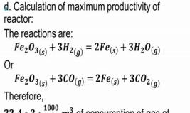
22.  $4*3*\frac{1000}{273}$   $m^3$  of consumption of gas at 1000K leads to production of 2x56 kg iron. Again, utilization of reducing gas is only 20%. Therefore,  $\frac{100}{20}*22.4*3*\frac{1000}{273}*m^3$  of gas is required to produce 2x56 kg iron.
