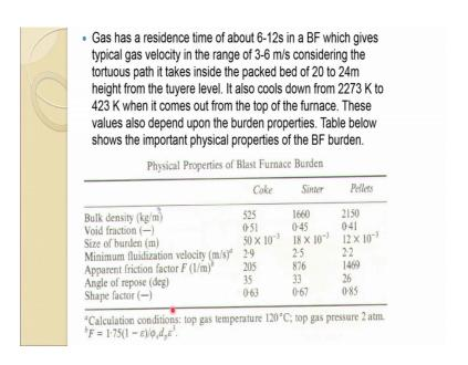
So, gas has a residence time of about 6 to 12 second in a blast furnace. We skip typical gas velocity in the range of 3 to 6 meter per second considering the tortuous path it takes inside the packed bed of 20 to 24 meter.
