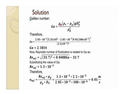
So, essentially you know the Galileo number you have to calculate Galileo number. So, Galileo number is you know it is given by this and do you know is these values you can substitute sort of Galileo numbers come to this. Now either you can calculate Reynolds numbers by substituting this Galileo number over here or you can even directly calculate from these it is you have the your Galileo number is about 2.18, so which is really somewhere here.
