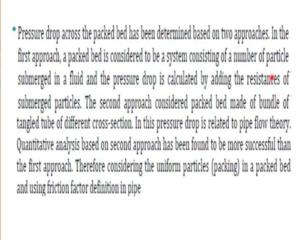
So, this is the one which one has to measure it in a packed bed. So, pressure drop across the packed bed has been determined based on 2 approaches. So, in the first approach a packed bed is considered to be a system consisting of a number of particle submerged in a fluid and the pressure drop is calculated by adding the resistance says a submerged particle.
