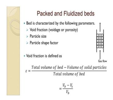
So, when we do replies the case gas from the packing in the container, there is a resistance offered by these particles to the gas flow packed bed. The resistance is offered by these particles to the gas flow. So, you will get if you measure the pressures here and here, you will see there is a pressure drop in this one which is the birth against this resistance.
