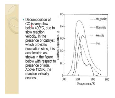
In the presence of catalyst which provides nucleation sites it is accelerated as shown in this figure and this is with respect to presence of iron so iron becomes as a catalyst and so this reaction is accelerated. So, above 1123 Kelvin, 900 degrees see the reaction virtually sees as we mentioned in this one above 9 900 degrees. See this is almost over this reaction does not occur that 1 so you can see the in the presence of magnetite carbon deposits is maximum.
