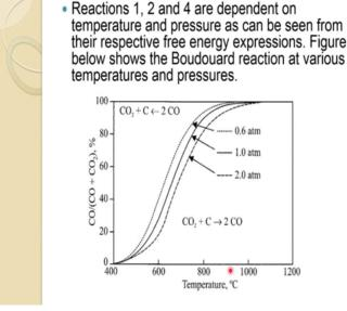
So, reaction 1 2 and 4 are dependent on temperature and pressure as we have seen with the free energy relation with respect to free energy expression. So, these can be plotted in graphical forms. So, figure below shows the bouldouard reaction at various temperature and pressure. So, this is bouldouard reaction carbon gasification reaction and one can see plotted temperature versus C O C O plus C O 2 ratio.
