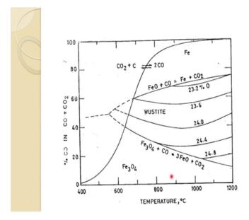
So, it has been superimposed and on the Fe C O system just to say how the deduction will take place. So, essentially Fe C O system is this one with these lines are there so
