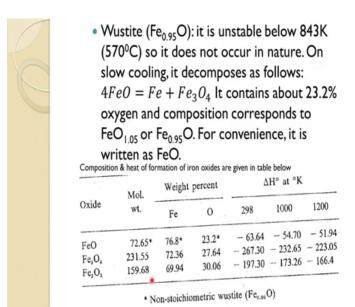
Now we have Wustite Fe O it is unstable below 843 3 p degree Kelvin that is 573 degree Celsius so it does not occur in the nature. So, once you know Fe O is not in naturally occurring compound because it is unstable. On slow cooling it decomposes as follows. So, it keeps actually magnetite and iron.
