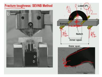
This is something we can measure, experimentally. How we can measure the fracture toughness? We can measure the fracture toughness by ACBMB. ACBMB stands for single H, V notch P. As the name suggests, it means we have to introduce V notch in one of the ages and that age is to be placed on the tensile surface. Now, once you produce the P notch on the tensile surface, then you have to break them into Flexural mode. This is 4 point Flexural mode.
