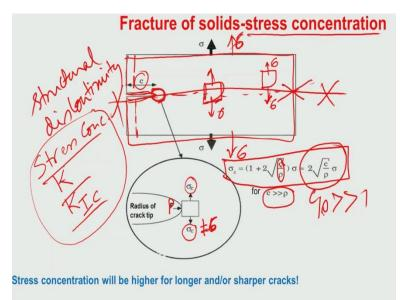
So, the three things that is important for one to remember. One is the stress concentration. Second one is the K factor that is the stress intensity factor. Third one is K1C that is the critical stress intensity factor, under mode 1 loading. So, this is more than enough just to understand many things which is required to know about the fracture of the brittle solid like bone and fracture of the brittle solids like ceramic best materials.
