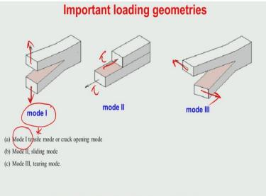
Mode I is the dangerous since the tensile stress is trying to open up the crack.
