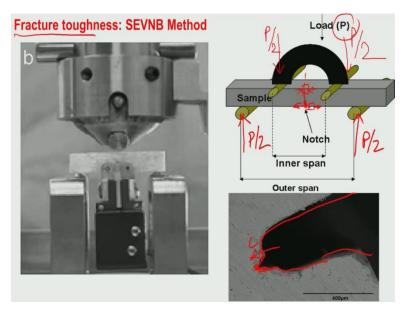
So, what you see here? This is a 4 point loading assembly. So, if you apply this is you P by 2, then the load is distributed at arms. So, this is P by 2, P by 2. And now what is the result put forth? There is P by 2 and P by 2. So, for every action there is equivalent and opposite reaction. So, if P by 2, P by 2 load is there from the top, so P by 2 load, P by 2 load, also would experience at the 2 rollers which are kept at the end of the outer span.
