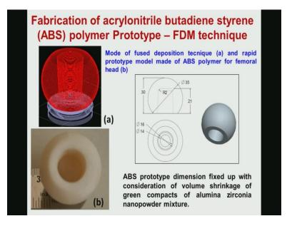
So, here again you have to first develop the mold where this ceramics is to be fabricated. And this mold essentially is made by that FDM technique which is the rapid proto typing technique.
