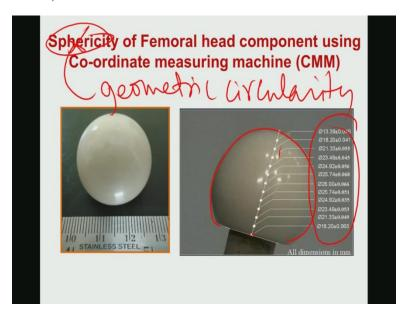
Now, this one has to measure the sphericity of this material so, geometric circularity that instead of sphericity that we also call is a geometric circularity. Now in this geometric circularity you can find out that what is the different dimensions of these materials and how this materials is polished and smoothly polished materials. And different points you can measure this and see that what is the design file and what is the product file what is the product file.
