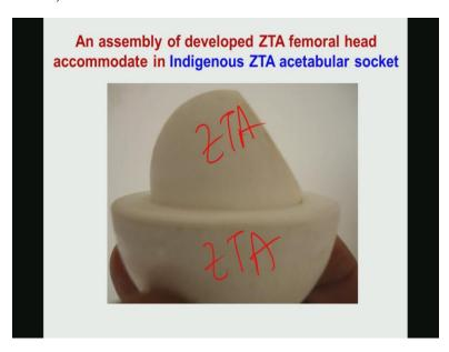
Now this is one of the assembly of the femoral ball head, this is the ZTA femoral ball head and this is the ZTA femoral socket. Now in the as fabricated without any machining in the Neoschip fabrication conditions you can see that what is the geometric conformity of this ZTA femoral head with acetabular socket. Essentially it shows that it is essentially a good conformity.
