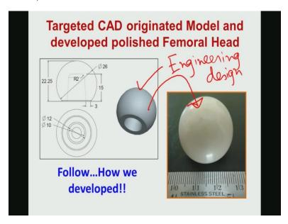
As I said that first eight for the prototype development is the engineering design. So, therefore I am showing you that what is that CAD file, CAD design file of this material design. And you can see that various dimensions that are mentioned and then ultimately your aim is to translate that design concept into the prototype product by certain intrigued manufacturing protocol.
