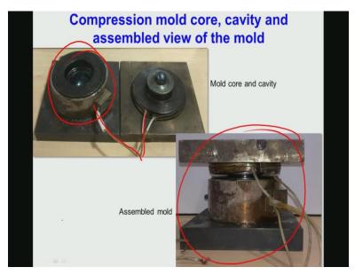
So, this part of the work can be was carried out in Central Institute of Plastic Engineering Technology, Chennai and this is through a heating coil arrangement. You can locally heat this entire assembly. But this heating requirement is fairly minimal unlike ceramics, so, here if you heat it at close to 200 or below 200 degree Celsius and it contain HDP that should be fine.
