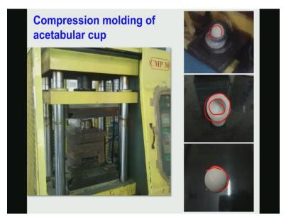
And this is how this compression mold socket that looks like and this is your as fabricated neon net shaped and so you don't need to do much machining or you don't need to do any machining to get the final shaped and this is kind of really elastration of the neon net shaped of fabrication of the acetabular socket.
