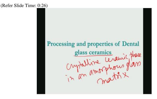
Now this glass ceramics is essentially defined as a materials which contains crystalline ceramic phase in an amorphous glass matrix. Now one of the things that I will be doing in this module is that first I will be briefly introduce to that dental implant systems to start with and then I will discuss rest part of this module only on the processing and properties of some of the machinable glass ceramics.
