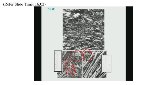
Now in terms of morphology what we see that this mica straw like crystals they are forming not only in one direction but also in different directions depending on whether this materials are crystallized or ceramized at 1000 degree Celsius for 24, hours.
