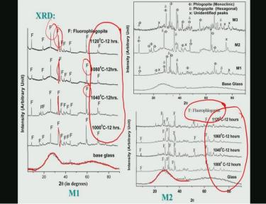
Now to illustrate further that ceramization process in this particular case was carried out at different temperature of 1000 degree Celsius to 1020 degree Celsius by holding them, by holding the glass at this different temperature for 12 hours. Now depending on what is the temperature that you are holding it for 12 hours, what you see that initially the glass has a very large hump and this hump essentially is a characteristics of any amorphous material.
