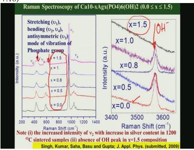
So Raman spectroscopy analysis further confirms that difference in stretching, bending and asymmetric mode of vibration of the phosphate group that has been shown here indicated by different arrow at different places and as you can see that this is also dependant on the different substitution level of the silver into hydroxyapatite.
