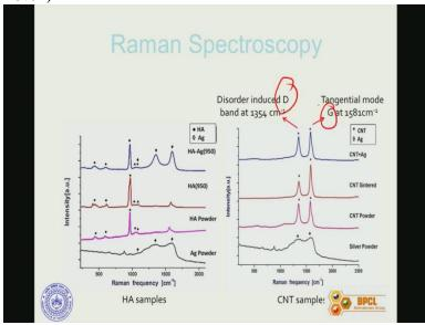
Then second one is the Raman spectroscopy analysis shows that particularly carbon that disorder peak and graphitic peak are clearly present at two distinct Raman bands of 1354 and 1581 centimetres inverse respectively.
