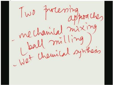
So the mechanical mixing and in both the cases, so two processing approaches. One is that mechanical mixing, so mechanical mixing essentially means that is the ball milling. And then second one is that wet chemical synthesis. Now wet chemical synthesis approach will be emphasised in this module. Now mechanical mixing simply means that you take hydroxyl powder and you take metallic silver powder, you mix it with certain for certain time with the
