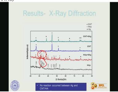
Now when you do this hydroxyl carbon nanotube and silver composites, so we have done classic material science analysis of X-ray diffraction just to confirm that characteristic hydroxyapatite peaks are retained in the spark pulmo sintered composites.
