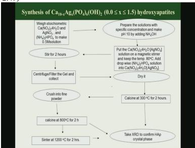
So like any other wet chemical synthesis you start with the precursor solution of this silver as well as the hydroxyapatite, and the precursor solution here is the silver nitrate for silver and then for hydroxyapatite we are using calcium nitrate. 4H2O(Ca(NO3)2.4H2O) and ammonium phosphate that (NH4)2HPO4 and then we make this 0.5 molar solution of this particular precursor, then you stir if for two hours then you centrifuge, crush it and then calcine it at 300 degrees for 2 hours.
