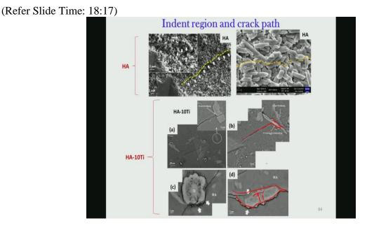
Now as far as the toughness is concerned the what we have observed that when you have titanium on the way this crack is going and then crack there is a evidence of the crack going debonding and crack breaching. And this is kind of very clearly, here you can see titanium here and around the titanium there is some evidence of the crack breaching as a additional toughing agents.
