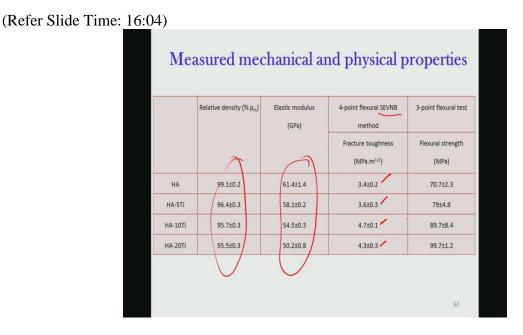
Now coming to the mechanical properties of these material, first of all these material are sintered more than 95 percent theoretical density. Elastic modulus also is fairly low. It is I mean although a little this is 50 to 60 giga Pascal. SEVNB, single edge v notch beam technique when you measure, this fracture toughness values are relatively high 4.3 MP square root meter.
