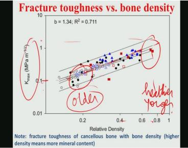
So bone density is also important in case of a natural bone and this essentially shows that this fracture toughness scales with the it goes bone density, so this is for the cancellous bone, it goes from .1 to somewhere above 1 mps square root meter. Now bone density if your remember, bone density essentially depends on the hydroxyapatite content or calcium apatite content in the in the natural bone. So higher the relative density of the bone means higher is the mineral content.
