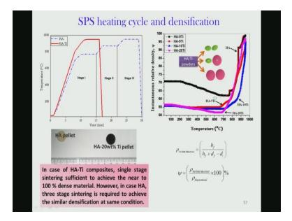
So what we do, we try to sinter them in spark plasma sintering in argon atmosphere at a temperature of 950 degree Celsius and so on. And then idea is that if you heat them very fast and if you hold them for smaller time period then you are not allowing the hydroxide titanium to react stop so all the conventional related sintering reactions can be avoided and you can achieve higher densification.
