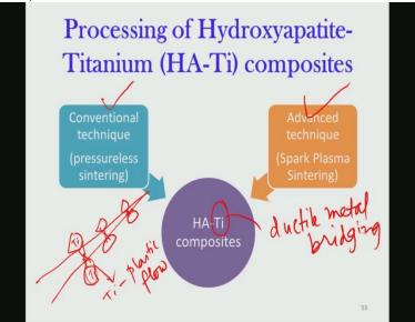
So what we use is the titanium as a metallic re enforcement. Now why titanium, because titanium being a metal, it can enhance the fracture toughness through the mechanism is ductile metal breezing. So ductile metal breezing essentially is a concept is that, suppose you have a titanium particle somewhere here and the crack is going to pass through this kind of micro structure.
