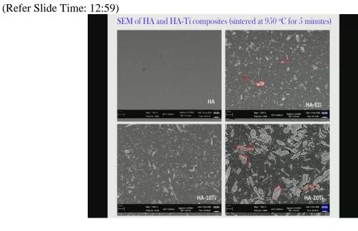
Now as far as the acm images of this titanium distribution is concerned, what you see that titanium particles are distributed quiet uniformly but at higher titanium quantity like 20 percent titanium and so on, you can see that there is a plaster of titanium particles which is distributed in the hydroxyapatite matrix.
