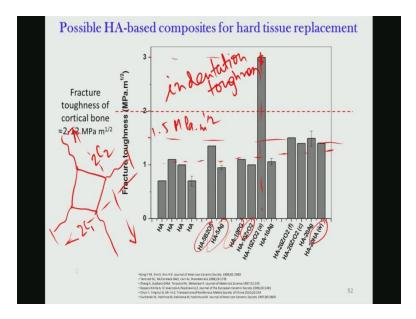
k. Now what is the driving force for development of the hydroxyapatite based composites in the bio ceramic applications? Essentially as I said that most of the hydroxyapatite based materials, if you plot their fracture toughness properties, what you see here, we have tried to summarize here. So this is B2o5 has been used as a reinforcement. Silver has been used as a reinforcement. Phosphate glass, zirconia and various other materials, hydroxide whiskers has been used as a re enforcement.
