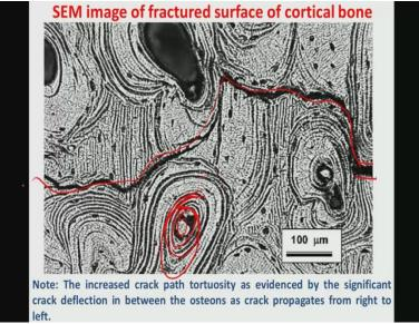
nd this is how the fracture takes place in the cortical bone. As you can see that we have introduced some v notch, then the cracks will go like this. In then this is your osteons. Different concentric circles and then cracks will essentially go through at the periphery of the osteon surface and go toward the other end of the bone structure.
