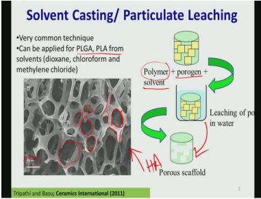
So, the solvent Casting or Particulate Leaching It is a very common technique. What you do here? You start with a particular polymer which is the base polymer. You use some porogen, this porogen can be some sacrificial agent, like, you know, Sugar, or kind of salt crystals, and all NaCl crystals and all. And then after you add this, then you put it in the water and then you see that how this Leaching takes place. And this Leaching is done, then it gives you a Porous Scaffold.
