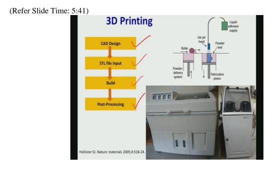
Now, in the 3D Printing Technique, again you start with a CAD Design, so that is computer aided design. You make the Stereolithography file as an input file. Then you have a build Piston and you have a Post-processing, okay? So in the Build Piston and Post-Processing, what you see here that how this structure is being built and then further how it will take a particular concept.
