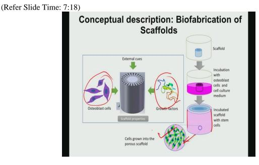
Now in more is the Tissue engineering applications like this is called Biofabrication. Why is the 'Bio'? 'Bio' word is used simply because you are using certain growth factors and then cells, together uh with that material itself from which you are making the Scaffold during the fabrication itself in situ. That means that with the help of growth factors and cells, Osteoblast cells like bone forming cells for bone tissue engineering, now these cells can be any type.
