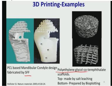
So, this is some of the examples of this 3D printer structure like Polycaprolactone-based Mandibular Condyle Design fabricated by Solid Freeform Fabrication. SFF stands for isolid Freeform Fabrication'. And also PEG Polyethylene Glycol based Scaffolds like Salt leaching and prepared by Bioplotting.
