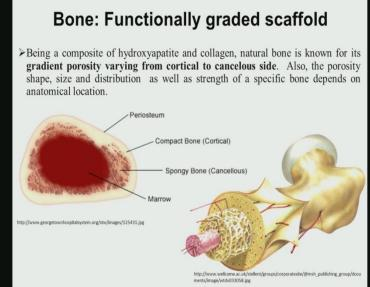
Now, in the context of biomedical applications. Um this additive manufacturing or 3D printing based techniques have received wider attention or have received uh have attracted lot of attention simply because that bone is a natural bio composite which is made of Hydroxyapatite and Collagen, and bone has different varying porosity in the structure. And this gradient porosity varies from cortical to cancellous side.
