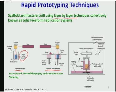
Now, coming back to the Rapid Prototyping Technique, the fundamental definition of Rapid Prototyping must include that layer by layer deposition technique. That is the generic description in whatever Rapid Prototyping Technique that you are using, whether it is for Scaffold fabrication for paramedical application or whether it is for structural applications like a dense component, non-porous component, everywhere these things is used.
