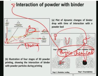
Some physicochemical interaction, physicochemical interaction essentially means that once your drop comes here, and then this is your powder base, the drops first to be wetted. So there should be wettability of the powder with that binder. Once it is wettable, then drops can be integrated into the powder bed and then this will dissolve. So it has to be dissolved like some chemical interaction. So this we call 'Physico-chemical interaction', ok?
