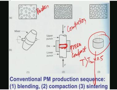
So this is that typical conventional parametrogilcal based processing of the ceramics. So you start with the powder first, so its a powder. Then you mix with some additives or you mix two different kind of powders of two different chemistry. Then you do this is called compaction stage. So this is first is the powder blending, then is the compaction, then you get this kind of small cylindrical shaped green body that is green, this is called green compact.
