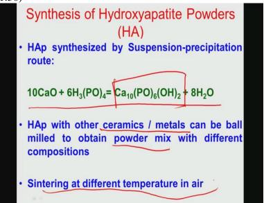
So one of the important process of sintering is that how you can make this powder that is what I said. So I will just give you an example of that hydroxyapatite powders. Because why hydroxyapatite, because hydroxyapatite again I recall that hydroxyapatite is the in organic constituent of the natural bone. So therefore hydroxyapatite powder how it is synthesized I have mentioned.
