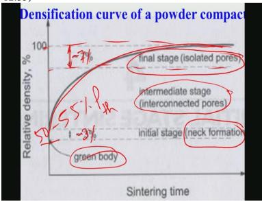
So this is what has been taken place that is the initial stage there is the neck formation. Intermediate stage that is the interconnected pore formation. And the final stage of densification that is the closed pore formation. So initial stage that is density changes almost 3 percent and your start with a green body which has the density something around 50-55% of the theoretical density.
