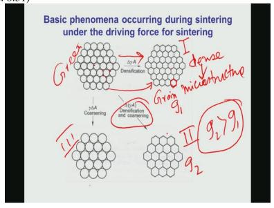
Now in case of basic phenomenon which occurs during the sintering is essentially what I have shown here. This is the spherical powder particles, now this spherical powder particles which,
