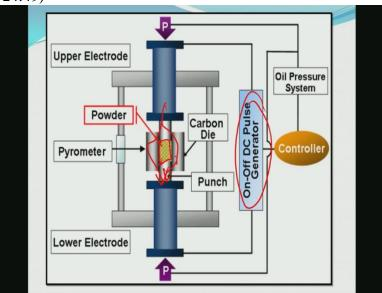
And in this graphite plates that this depending on the conductivity of the sample powder and depending on the conductivity of the graphite dye punch assembly, some fraction of the current will go through and this is a very clear picture. Like you can see that powder particles here and this is the fraction of the current will go through like this. And this fraction of the current will go through and this is the DC pulse generator and then after that what will happen?
