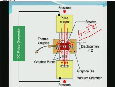
Depending on how much current is passing through the powder compact, powder compact will be heated up. So this T is heating is typically done by the Joule is heating where h is equal to I square rt. I is the current that is flowing through the sample, r is the resistance, that is conductor resistance and t is the time through which this current is passing through the material.
