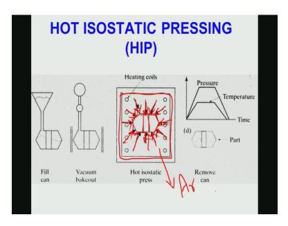
What is the advantage between, of hot Isostatic pressing over hot pressing? Now if you look at hot pressing technique which I will come to here, so in the hot pressing, you put the ceramic powder or for that matter of fact any powder particles. Then it is a external heating process. So the heat is coming from outside through inductive heating coil and that temperature can go up to 1800-2000 degree Celsius. And then when it becomes red hot then you also apply compressive presser here.
