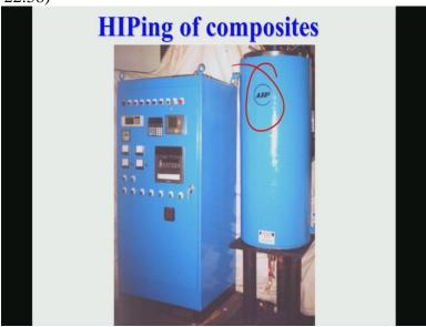
So therefore little bit more details of the hot Isostatic pressing. This is the American isostatic press, this is aip, stands for American isostatic press, who manufacturers this kind of isostatic pressing.
