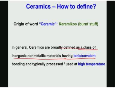
So the word ceramic essentially is derived from the Greek word ceramico that is bond stuff. And in general ceramics are defined as a class of in organic non metallic materials having ironic covalent bonding and typically processed or used at high temperature.
