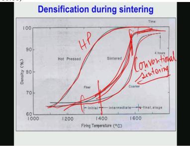
This is a typical sintering curve like how the density changes with the sintering temperature. Now what you notice here that all this curve has a similar qualitative description. Like this is a finer particle powder, this is a coarser particle powders and this is the hot pressing. What is hot pressing I will come to this in after 5-10 minutes. So hot pressing is a unique technique where you are applying uni axel compression pressure when you are heating the powder compact.
