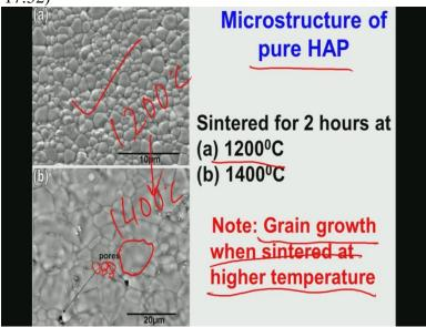
This is the classic example of hydroxyapatite micro structure and what you see is a very fine scale micro structure which is sintered at 1200 degree Celsius. Now what I'm showing here this is 1200 degree Celsius sample. And this is 1400 degree Celsius if you compare immediately between this and this, what you see there is a large grain size and there is a small number of grains also here. So this is the smaller grain size and this is a much larger grain size.
