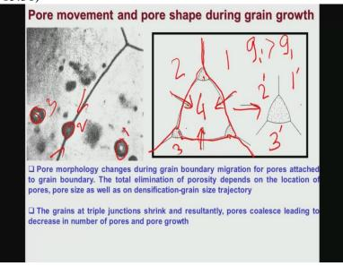
So as the sintering process advances, what happens is that when the pores will not be any more connected to each other they become isolated. Then that particular case it is very difficult to remove the pores. Because I will just give you the three examples one is the pore number 1, one is another pore number 2 and third one is pore number 3. Here pore number 1 and pore number 3 are located well within the grain. Pore number 2 are located at the grain boundary region.
