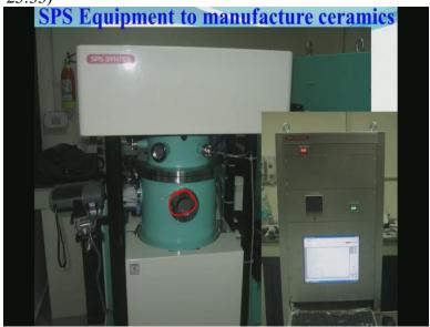
So because of this high pulse current, now you can see through this window that how this temperature is going, shooting up, this is a commercial spark plasma sintering machine, where hydroxyapatite based material can be routinely consolidated and densitfed and then you can do this sintering process and you can sinter it even at higher temperature to consolidate the material.
