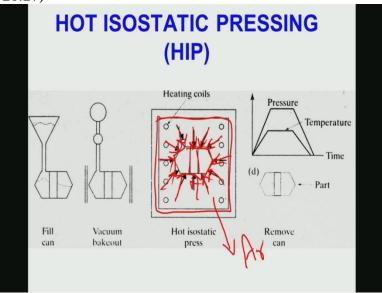
So one of the most advanced sintering processes is called hot isostatic pressing. As the name suggest hot isostatic pressing means you are applying equal pressure from all directions. Now the classic example is that, this is a typical hot isostatic pressing chamber. So we fill it up with some high pressurized gas let is say argon, so argon then you pressurize it like 300 mega Pascal and so on. And then you put your sample somewhere here, in a glass container.
