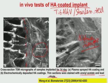
Ok, these are some other examples, which is shown for hydroxyapatite coating. Remember this hydroxyapatite coating is widely used on the major orthopaedic implant alloys, like titanium 6 aluminium 4 vanadium or 316 L stainless steel stem. So this hydroxyapatite coating depending on the way these coatings are deposited on the substrates whether it is called electrolytic position or whether it is called plasma spraying.
