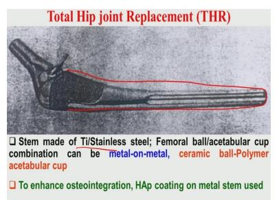
Now total hip joint replacement is one of the popular example of titanium stainless steel is used as the stem. Nowadays one of the developments is that one can use hydroxyapatite coatings on this titanium or stainless steel structures to make it more biocompatible on to have better osseointigration properties.
