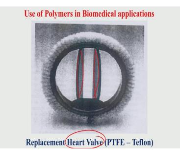
Cardio vascular applications, this is a very popular example of heart valve, this poly tetra fluoro ethylene so it is used for blood contacting devices do therefore thrombogenesis is one of the properties one is to check for.
