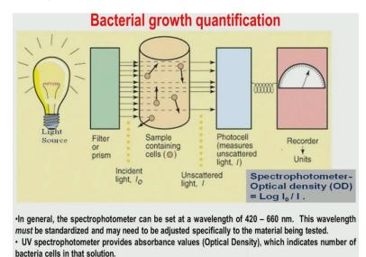
Now how you can quantify these kind of growth kinetics, 1 of the most standard and widely used method is Spectrophotometer, as the name suggests that means that there is certain light where (ba ba) light ray of certain wavelength will be made to pass through the bacterial growth medium. Once without bacteria and once the blank solution like that is the blank solution and 1 case with bacteria, actual growth medium containing bacteria.
