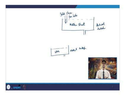
So, if you try to see that you will have suppose, in the case of your actual tundish may be like this. So, you will have in this case you have the molten steel here and you will have the level of steel suppose here and then inlet is from this side so, your molten steel is flowing. So, you will have inlet stream from ladle.
