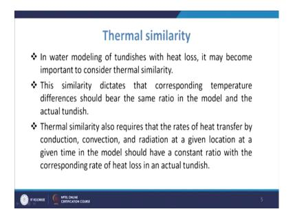
So, when we talk about the water modeling so, normally in water modeling you know when we do for the tundish. So, with that the heat loss you know which is taking place at that high temperature so, its very difficult to correlate. But then we will have we can have this thermal similarity and what we can do is here also whatever the temperature difference is there suppose, if they are in the same ratio then we can say that the systems are thermally similar.
