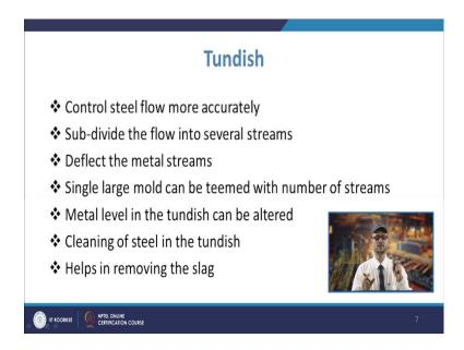
So, basically you have you know this way it controls that you know the I mean quantity of metal which is flowing into the mold. Now, coming to talk about the dividing the flow into several stream. So, what happens that when the flow will be coming here and when it will be striking; so metal will be going from here like this and it will be going like this from here. So, this way it will be moving to in the different streams, the metal will be going.
