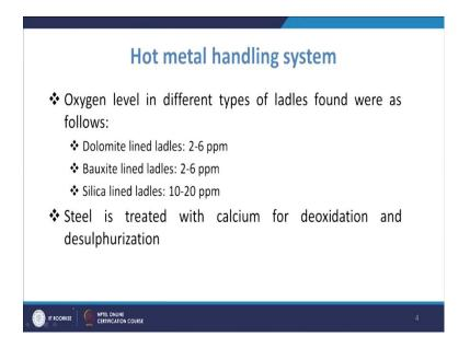
Now, steel will be treated with the calcium for the deoxidation and desulphurization. So, in most of the cases, we tried to have the minimum amount of oxygen as well as sulphur is also deleterious for the quality steel. So, we also try to treat with the calcium for the deoxidation and the desulphurization. So, that is what is normally the practice for the you know in the industries by using the calcium.
