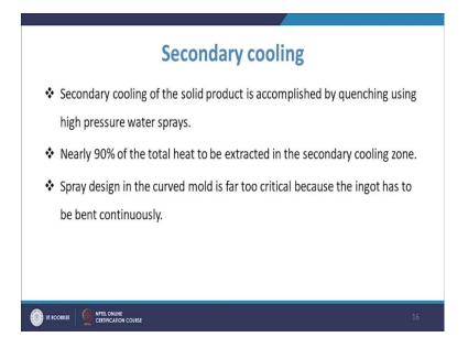
After that you have the secondary cooling of the solid product and it will be accomplished by quenching using high pressure water sprays. So, we are using those hotter water sprays and then, require the cooling is done.
