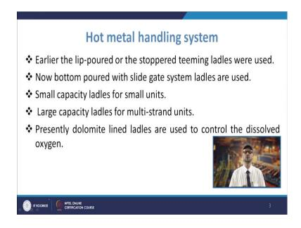
Coming to the hot metal handling system. So, as you know that it brings the hot metal and it its job is to pour it into the tundish. So, earlier the lip poured or the stoppered teeming ladles were used. So, that was the practice earlier, but now most of in most of the cases bottom poured with a slide gate system you know ladles are used.
