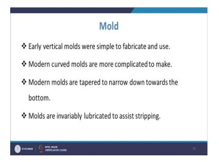
So, you have earlier vertical molds, then you we get nowadays the curved molds which are complicated and modern molds are tapered to narrow down towards the bottom and its basically to account for the shrinkage. Because when we know that you know there is tapering which is done because the metal which is getting solidified and it has a higher density. So, there will be shrinking of the metal and to account for that there is some taper which is given you know the in the mold to account for that.
