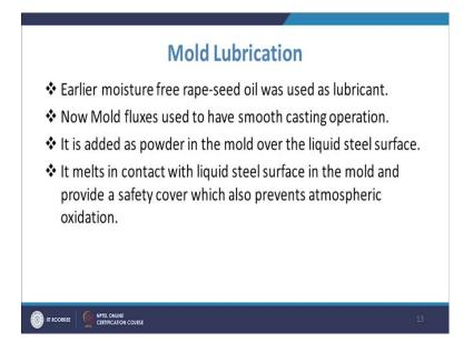
Now, we have mold fluxes are used to have these smooth casting operation and it will be added as the powder in the mold over the liquid steel surface. So, we. So, there is a normal practice you have a powder which will be given out the surface.
