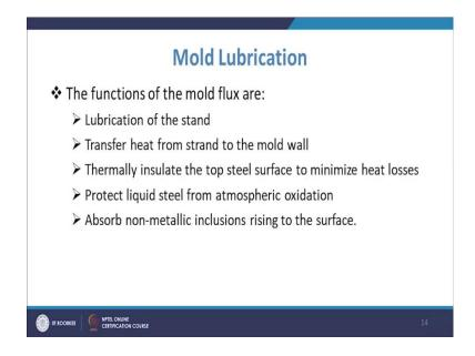
Then, the function of these mold flux are that there will be lubrication of the strand. Then, you have transfer heat from the strand to the mold wall and then, thermally insulate the top steel surface. That is what we have discussed.
