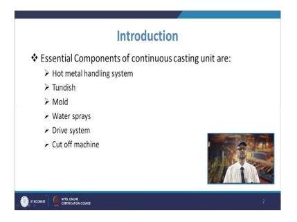
So, as we move on we will talk about these following components like a hot metal handling system, then you have tundish, mold, water sprays, drive system and then cutoff machine. So, all these you know system, all these components make one continuous casting unit and a hot metal handling system is it will start from the you know that system which will be handling that hot metal, it will be bringing that hot metals that is especially the ladle.
