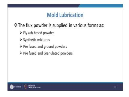
And they are in different forms, we use it like fly ash based powder, synthetic mixture, pre fused and ground powders and then, granulated powders also. So, that way we give these more lubrication.
