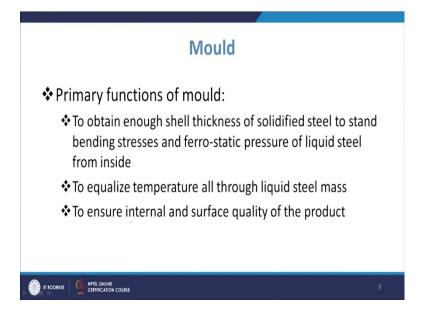
So, if you talk about the function of the mold, it is to obtain the enough shell thickness of solidified shell to stand bending stresses and ferro static pressure of liquid steel from inside. So, what we see nowadays we have seen that also you are mold is from there itself, it is somewhat curved. So, you will have the bending stresses and also you have the ferro static pressure of the liquid steel.
