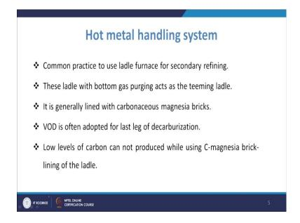
Common practice to use the ladle furnace for secondary refining. Now, what we have earlier seen that nowadays it is a very common practice to use the ladle furnace. So, that is a very important tool for the secondary refining process and in that basically you have these ladle, with the bottom gas purging. So, you will have the purging from the you know bottom the gas purging is done and that acts as the teeming ladle.
