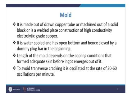
So, then you know the metal comes towards the mold. Now, we all have already discussed that we these mold is made of the drawn copper tube or machined out of a solid block or is a welded plate construction of high conductivity electrolytic grade copper.
