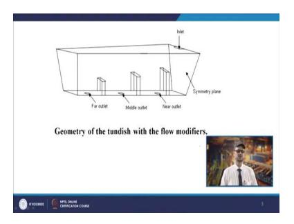
So, we and that is also a published work. So, in that how we make the geometry. So, in the geometry you have inlet, you have a symmetry plane. So, it is basically a six-strand; you know tundish and we also have used these flow modifiers. And this is the near, middle and far outlet from the inlet. So, that is why we have named it like that and this is the symmetry boundary condition and this is the inlet through which the inclusions are also you know may insert it or allowed.
