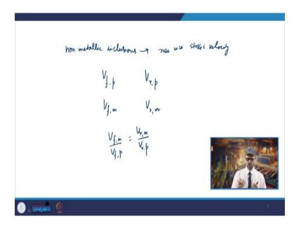
So, these nonmetallic inclusions, so, they rise with stokes velocity. It is just assumed that they rise with this absolute velocity. So, you have the velocity of the fluid also and then you have the rise velocity. So, if you talk about the velocity of the fluid and in the prototype, so, we call it as velocity of fluid in the prototype that is and in the prototype tundish. Similarly, you will have the velocity of the rise in the prototype tundish.
