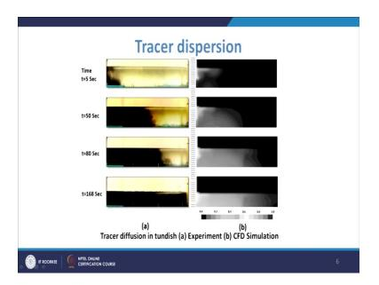
So, this is just showing one example of these Tracer dispersion and what you can see that this is the experiment. So, you gave the you know this is how the flow is going on with
