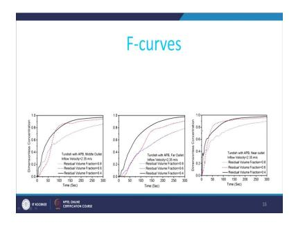
So, residual volume fraction if it is a smaller than a smaller that will be leading to the lower value of the intermixed amounts, that is what is seen you know even with the use of APBs also you can have that feeling.
