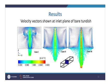
This is the velocity vector which is you know showing that how you are increasing the you know velocity for the three cases. In one case it is about 1.78, then it is increasing accordingly.
