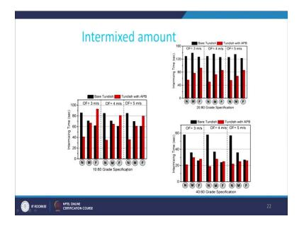
So, basically thing is that you can have the different parameters changed and accordingly you can calculate the intermixed amount. And you can suggest in the plant that if you maintain this flow rate or if you have the proper selection of these of process parameters, in those cases you are likely to have the minimum of the intermixed amount. And the decrease in the value of intermixed amount will basically increase the productivity of the plant.
