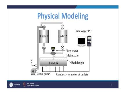
So, if you try to do the modeling physically what you have to do is, you have to have two ladles and you have a flow meter and then, you have the inlet nozzle here. So, you allow these liquid steel to allow, so you will have the two type of fluid and one you can you know color and another you can be it can be white or so or different color.
