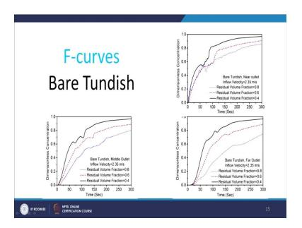
So, if you what is that effect on the residual you know volume and the ones having the residual volume means when the height is remaining at that particular volume fraction of 0.4 then you allow. In that case, when it is 0.6, then you allow or when it is at 0.8 of height then you allow means when you are allowing the new grade of steel to fall at that time, what is the height of the steel of that old component in the tundish.
