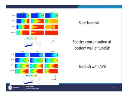
So, this is about the species concentration that you can draw and you can see that with time how your you know concentration is increasing. So, from inlet it is increasing towards the. So, as the time is increasing how this tracer concentration is going to change after at the time is progressing and you can see that if you increase the flow, then that case how it is
