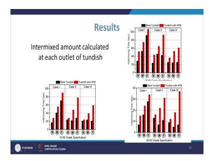
So, that can be calculated. So, once you you know calculate for a particular kind of grade specification suppose for 10:60 for 20:80 or 40:60 grade specification, these data's can be you know calculated and they tell that if you go for case 1, you know where the you know flow of the velocity was same and in this case flow was you know increase in case 2. Case 3 was you know further increased.
