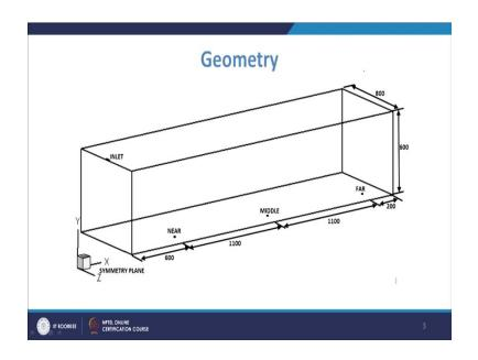
So, on this I had done this simulation. So, in that what we see is that this is a typical tundish and as you see that this is the inlet and these are mid NEAR, MIDDLE and FAR are the outlets. So, this is typically a multi strand tundish you have more than one outlet.
