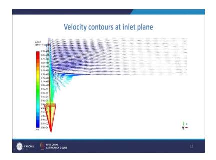
So, as you see these are the velocity contours at the inlet plane and this is the velocity if you look at the inlet plane as you see this is the inlet vertical plate. So, as you see that you have the flow which is coming on the coming in the bottom direction and then, it is moving from here. So, that way and it is moving through here and then.
