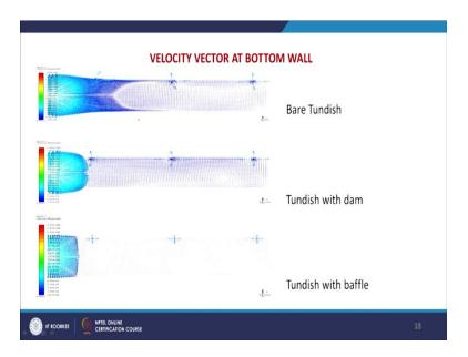
You can also see the velocity vector at the bottom wall. So, as you see that in the case of bare tundish its going like this; but in the bottom wall, you are at the bottom you see the
