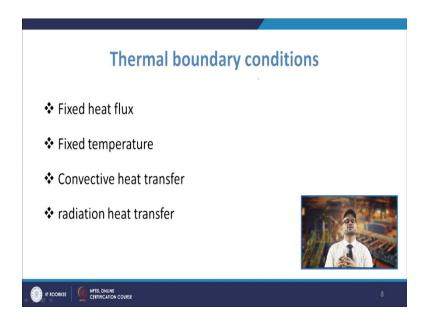
Now, the thermal boundary conditions are important because while dealing with these thermal boundary conditions you need to know that what should be the condition proper condition you should be selected. Like you may go for the fixed temperature kind of condition where, you say that the walls are at a fixed temperature and accordingly because the fluid is there inside the domain and the walls are at a fixed temperature.
