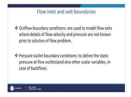
So, the outflow boundary conditions are used to model the flow exits for details of flow velocity and pressure are not known prior to the solution of flow problems. So, basically in normal case when you are defining the inlet velocity you do not know what will be the velocity at the pressure. So, you give the outflow boundary condition and this is the normally by default boundary condition given. So, it will you know take that depending upon the conservation rules.
