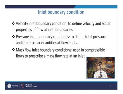
Now, the most important is the or every each one of these are important. So, first we will start with the inlet boundary condition. So, inlet is that place through which the medium you know of flow that will be moving and it will be going into the domain. So, there you need to have the condition. Now, in that you may have to specify a velocity and then you have a scalar properties of flow and the inlet boundaries.
