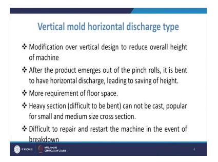
Coming forward you have another kind of you know design of the you know mold or the strand. So, that is a vertical mold and the horizontal discharge type. So, what we do in these cases; we have the vertical mold, but discharge is taken in the horizontal direction. So, cutting will be taken, cutting will be done you know when the slab or the billet is moving in the horizontal direction. So, you are cutting it.
