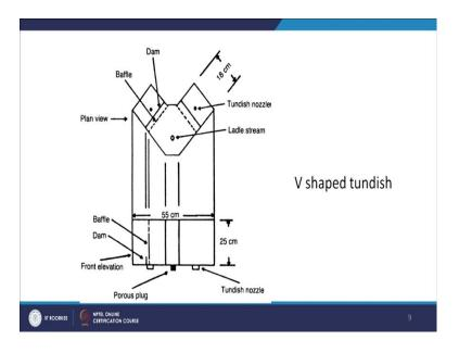
Now another design which is also popular in the case of a tundish is the V shaped tundish. So, you have a tundish which is of V shape, so it will come and then you have an angle. So, this angle, on this angle this shape is there.
