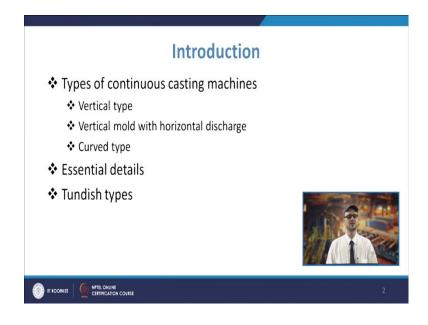
So, coming to the you know content in this lecture; I must tell you that this is we are going to discuss about the types of continuous casting machines. So, they are normally vertical type or vertical mold with horizontal discharge and also curved type.
