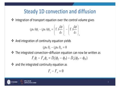
So, if you try to write these do the integration over the control volume, in that case what will happen this  $(\rho u A \varphi)_e - (\rho u A \varphi)_w = (\Gamma A \frac{d\varphi}{dx})_e - (\Gamma A \frac{d\varphi}{dx})_w$ . So, that is what this equation needs to be solved.
