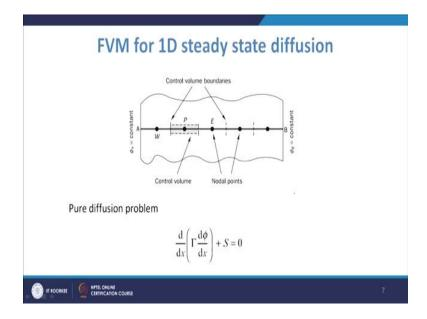
Now, what we see that how we have to know that how this control volume method works. So, because when we are taking a domain in most of the cases, we will be solving the problem in 2D or 3D, but just for understanding, we will start with one-dimensional problem and also the two-dimensional problem.
