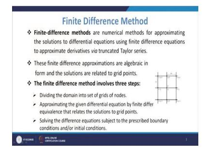
So, the finite difference methods these are the numerical methods for approximating the solutions to differential equations using finite difference equations to approximate derivatives via truncated Taylor series. So, basically what is required is that most of the these equations where you see these derivatives are there or there the differential equations, and we need to have the solution of these differential equations.
