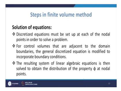
Similarly, I mean we can go for the, so what we see normally in the finite volume method, you have the discretized equation which is must be set at each of the nodal points in order
