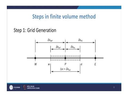
So, what we do is initially we go for the grid generation, and as you see that if you take any point P, so what happens on the, so on the this is the control volume. So, what you see this is the east phase of the control volume, this is a west phase of the control volume, and this is the grid node P.
