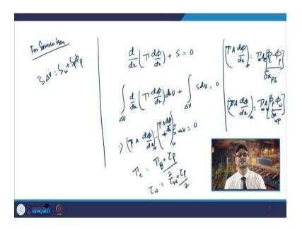
Now, how we get the equations in this form, so what we have seen we saw that you have  $\frac{d}{dx}(\Gamma \frac{d\varphi}{dx}) + S = 0$ . So, this is your equation. Now, if you go for the integration of over the control volume, so what you do is you are doing the integrations, you do the integration
