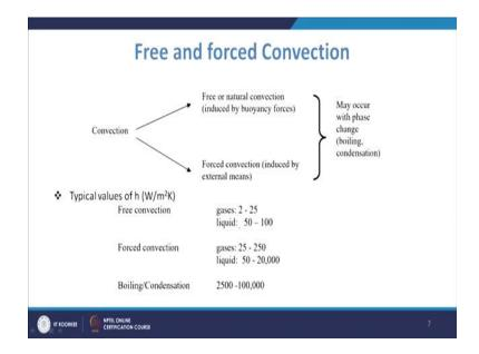
Now, what we need to know that when we talk about the convection, then there are two types of convection mechanism; one is the free or natural convection and one is forced convection, which is induced by the external means. Now, in the case of free or natural convection, you know what happens that because of that so that is basically induced by the buoyancy forces and it is basically in those cases when there will be change in the density.
