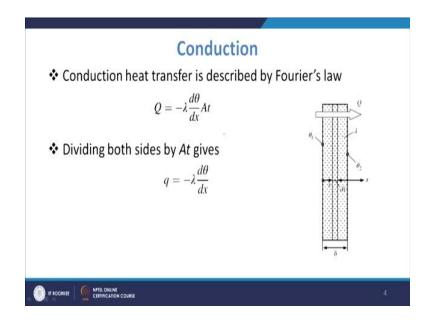
So, in the in conduction normally, now we use the Fourier's law of heat conduction and basically what has been seen that the heat transfer which is there, it will be proportional to the temperature gradient, then area and also the time. So, if you talk about. So, this is  $d\theta$  is nothing but the theta 2 minus theta 1 is if you have you know a reason, that is the higher temperature side and this is a lower temperature side.
