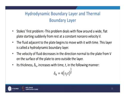
So, normally there has been the description of the hydrodynamic boundary layer and thermal boundary layer by dealing with the stokes first problem and where it is dealt that the you know you know there will be flow around the wide flat plate which is suddenly moved from rest to a constant velocity and then, what will happen that the fluid which is
