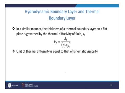
Now, in the same manner, you can have the thickness of the thermal boundary layer also on the flat plate and that is governed by  $K_f$ . The properties  $K_f$  that is your thermal diffusivity and that is  $\frac{\lambda_f}{\rho_f c_p}$ .
