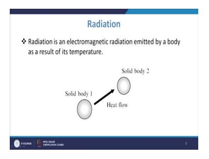
Then, you have another you know part is the radiation. So, radiation is again it is an electromagnetic radiation whereas, it is emitted by the body as a result of its temperature. So, in that case what happens that you have a body which is at higher temperature. So, it will be emitting the radiation towards the body of lower temperatures. So, that is the principle.
