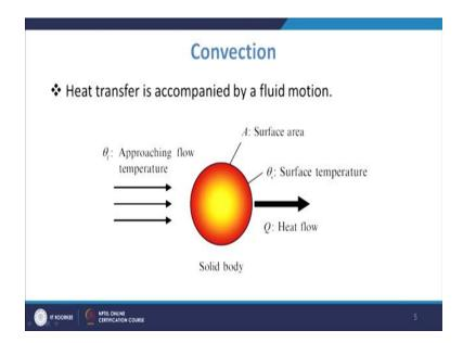
Now, coming to the convection. So, in conduction, we know that we need to have the value of the thermal conductivity and this is the property of the material and that will be required to have the value of the conductive heat flux or conductive heat you know which is transferred heat transfer by conduction. Now, heat transfer is also accompanied by the fluid motion.
