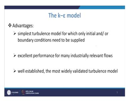
Now, the thing is that if you talk about this model. So, this model is basically a very you know simple turbulence model which is used for which only initial and order boundary conditions need to be supplied. So, we have certain name initial and boundary conditions suppose at inlet we give the distribution for k and epsilon.
