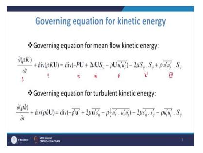
Now, for you know finding the equation for the mean turbulent kinetic energy you we had the equation you know for the you know for this mean component of velocity. So, what you can do is in that particular equation you multiply that with the mean component of velocity. So, that capital U and capital U will be U square. So, you will have 3 equations for that you know ah mean you know x component y component and that component momentum equation if you recall.
