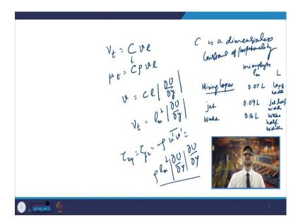
So, you know what is done is normally. What we see that  $v_t$ ; now in this you can write as the velocity scale and the length scale. So, because  $\mu_t$  has the unit of meter square per second, so you know this is meter per second and meters so it will be meter square per second. So, if the one velocity scale and one length scale that is described the effect of turbulence. So, in that case the dimensional analysis will yield to this equation  $v_t$  will be cvl.
