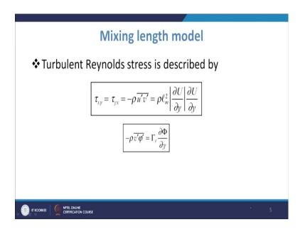
So, what happens you know in this case the turbulent stress I know. This is turbulent Reynolds stress what we do is we describe it in the form of this  $l_m^2$ ,  $l_m^2 \left| \frac{\partial U}{\partial y} \right| \frac{\partial U}{\partial y}$  here. So, basically what we see its expressed in terms of this I m, and then that is why you know we call it as a mixing length. Know its value also varies, so I mean there are certainly certain deviations for that.
