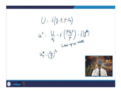
So, in that case your  $U = f(y, \rho, \mu, \tau_w)$ , now this $\tau_w$  is the wall shear stress in this case. So, this is basically for the close to the wall and when you do the dimensional analysis in this case then what you see is that the dimensional analysis will show that you get  $u^+$  that will be equal to  $\frac{U}{\mu\tau}$ .
