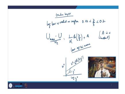
So, if you go to the outer layer. So, you know the log law of layer that is shown to be valid experimentally in the region. So, log law will be valid in region. So,  $\frac{y}{\delta}$  so, in that value has to be more than 0.02 and less than 0.2. Now for the larger value of the y the velocity defect law which we have got that gives you the correct you know form and in the overlap region basically you have the log law and the velocity defect law that has to be equal.
