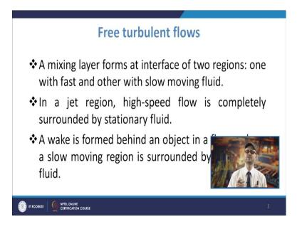
So, if you see the free turbulent flow so, in that case you will have 3 kind of you know flows. So, if you talk about the mixing layer. So, the in the mixing layer basically a mixing layer will be forming the interface of two regions: one with fast and one with the slow moving fluid. So, that is how they the mixing layer is defined.
