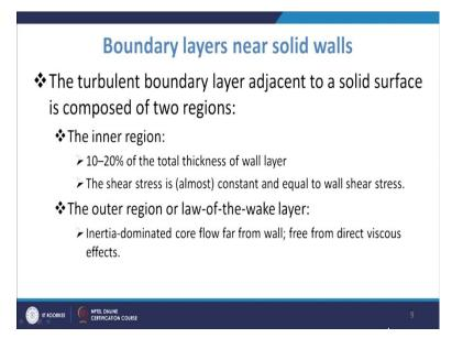
So, if suppose we are taking the case of boundary layer the near the solid walls. So, you know in the turbulent thin shear layer flows this Reynolds number based on length scale L in flow direction that is  $Re_L$  is always very very large. So, if you are taking that you know length scale L and if you are measuring that turbulence value this Reynolds number value that will be always very large and it that you know implies or; that means, that the flow is very much inertia dominated.
