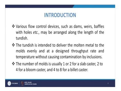
So, as we discussed that you will have the various flow control devices like dams, weirs, baffles with holes which will be arranged along the length of the tundish. And they are basically controlling the flow inside the tundish and you know you can understand it by you know process like if suppose you have a tundish.
