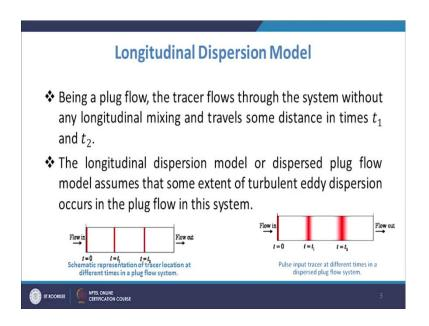
Whereas, when we talk about the dispersion model so, in the longitudinal dispersion model you know in that the tracer will flow through the system with certain longitudinal mixing. So, in plug flow there is no longitudinal mixing and travel some distance in time  $t_1$  and  $t_2$ . So, as you see that it will be you know it may t=0.
