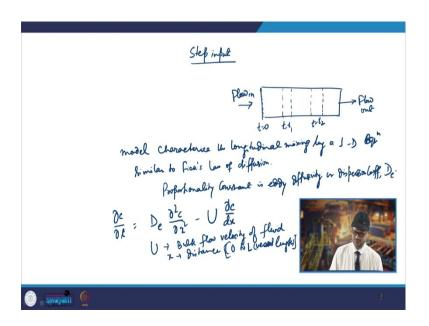
So, that was the case in the case of pulse input, but if you go for the step input also. So, in the case of step input if you see if you are you know you know flow is like going here. So, this will be flow in and this you will have the flow out. So, in that case also if you.
