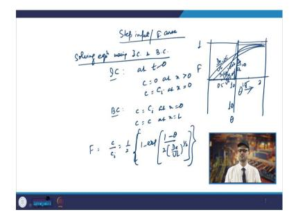
So, if you talk about the F curve. So, if you take the step input or F curve. So, the equation which we have seen earlier this was the equation. So, this was the concentration equation now this equation you know can be solved and you will have to have the initial as well as the boundary condition.
