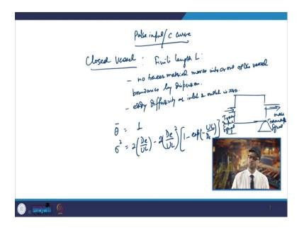
Now if we try to see for the pulse input so, if you go for the pulse input or you analyze the C curve. So, we have to further solve that equation that is  $\frac{\partial c}{\partial t} = D_e \frac{\partial^2 c}{\partial x^2} - U \frac{\partial c}{\partial x}$ so, that was this equation.
