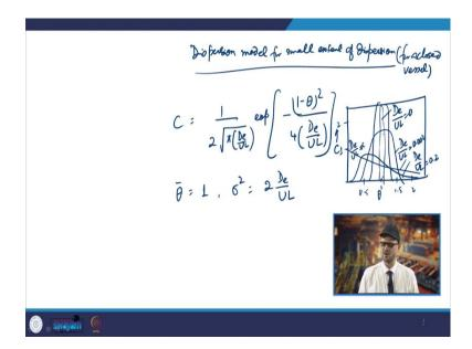
So, dispersion model for small extent of dispersion. So, where there is a small dispersion so, in that case what happens and for a closed vessel so, the closed vessel which is normally for the case of tundish flow. So, in that case the C curve is normally having a Gaussian type of you know profile. So, Gaussian type of RTD will be there when you have a low dispersion and small dispersion in the.
