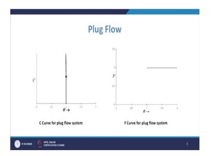
So, if you talk about plug flow system and if you talk about the C-curve. So, in the C-curve how can you schematically represent? So, what you see in the C-curve what you have seen that in the C-curve what you do is you give the sort pulse of tracer, it will go into the tundish and then it will come it will go inside the tundish at different location and then it will come to the outlet.
