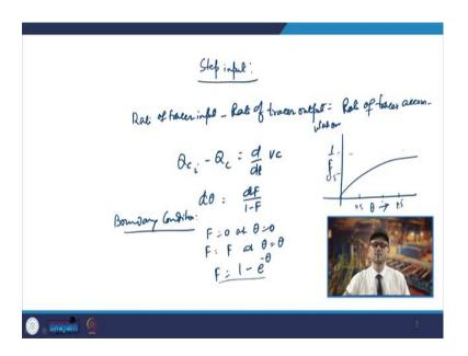
So, suppose we are talking about the step input. So, you have seen that in the case of step input for the plug flow it has there is nothing till t=0=1 and then your concentration value is dimensionless concentration value is 1, altogether. Whereas, if you talk about the step input case you know for the well mixed flow. Now, in that case you know again you can have the analysis like you have the rate of tracer input and minus rate of tracer output. So, that will be rate of tracer accumulation.
