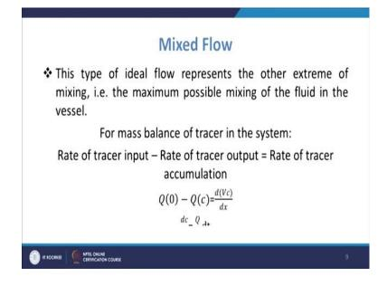
Now, next will be your mixed flow. So, the mixed flow will be the type of ideal flow that will be representing the other extreme of the missing. That is you know the maximum possible mixing of the fluid you know inside the vessel. So, to talk about the mixed flow, so in that case what we assume is that in a plug flow they are maintaining its identity whereas, in the mixed fluid is assumed that once that tracer has gone inside the vessel it has completely mixed inside.
