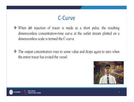
And the resulting dimensionless, so that results into dimensionless concentration. And time curve at the outlet stream and the curve which you plot for the dimensionless concentration and the dimensionless time that is C-curve and it will rise to some value and then drop again to 0 when the entire extra cell has exited the vessel.
