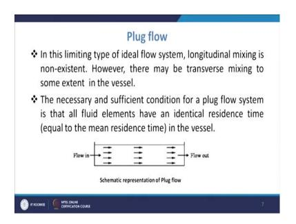
So, plug flow is; so in this type of limiting type of ideal flow system, the longitudinal missing is non-existent. So, what you see that normally you know we define as the metal which is the tracer which has gone. So, the plug flow means, the longitudinal mixing will be non-existent. So, the mixing in the longitudinal direction that is not at all there. So, it will have will be maintaining its identity and it will flow in you know on its path.
