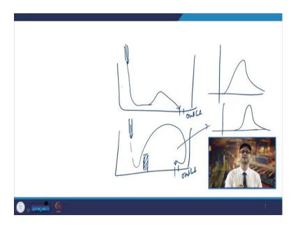
So, if suppose you have a tundish like this and in one case you have put in the tundish so, this is your inlet. So, this is from where the liquid steel is coming. Now, in this case and this is your outlet so, suppose this is the outlet, now the thing is that when you are basically giving the pulse you know that is tracer from here.
