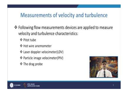
So, apart from that you will have the different flow measurement devices are applied to measure the velocity and turbulence. And in that you have pitot tube, you have hot wire anemometer, laser doppler velocimeter, the PIV is very much used in the case of physical modeling, where you try to have the you know velocity profile at certain section, so drag probe. So, these are the different you know ways by which you measure these you know velocity and flow profile.
