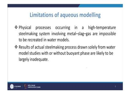
Physical processes occurring in a high temperature steel making system involving metal slag gas are impossible to be recreated in water models. So, as we discussed that it is very difficult to have the recreation of that system which is in actual present in the steelmaking case like you have the metal, then you have the slag and also you have the gas. So, it becomes a three phase kind of system which is nothing but the multi phase system, and you cannot make in water models.
