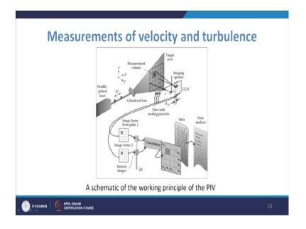
So, this is how your velocity and turbulence and PIV setup looks like. So, in that case you find the, you know the velocity profiles inside the vessel. So, this is about the, you know physical modeling aspects, the issues and challenges with that. And when we talk about the case studies and when we talk about other aspects, then we will have further you know discussion about these topics and we will have a more clarity in our, you know understanding.
