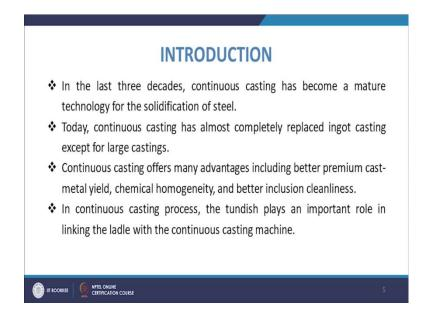
So, it has become a mature technology for the solidification of a steel and it has today almost completely replaced this ingot casting except for very large castings there we go for it, but otherwise we have completely replaced this process with continuous casting.
