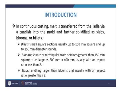
Then you know in so, coming to now the definition of the continuous casting. So, in turn continuous casting melt is transferred from the ladle via a tundish into the mold and further solidified as slabs blooms or billet us. So, what happens that in the case of continuous casting you have a ladle. So, this will be the ladle which will be getting the liquid steel.
