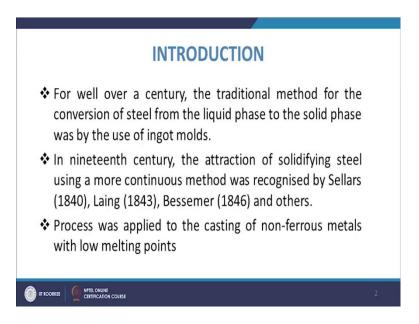
So, for well over a century, the traditional method for the conversion of steel from the liquid phase to the solid phase was by the use of ingot molds. So, as we discussed that in normal you know casting process, you have a conventional mold, you have a finite sized mold you know small size mold and you try to pour you know by from the furnace with some mechanism you pour the liquid metal into that mold and then you allow it to solidify.
