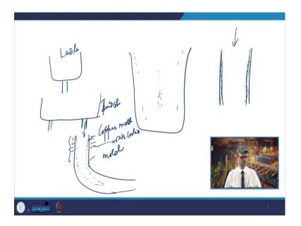
Now, once solidified once it is a so, there are solidification will start from all the sides this way and then this ingot will be taken for the further processing this ingot will be taken to the slabbing mill, that it will be going to the rolling mill, you have hot rolling then you have cold rolling. So, there are many processes which it has to undergo.
