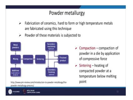
So, in case of Powder metallurgy alloys in this basically ceramics that can be processed only using Powder metallurgy processes or if you have material which are hard to deform or will have high temperature with their melting point is very high.
