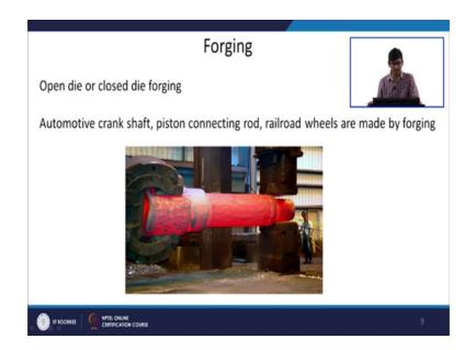
And you can see the size of the rolling size of the forge machine and the size of the material which is being forged ok. So, if you have Automatic crank shafts, piston connecting rods, railroad wheels are made by forging.
