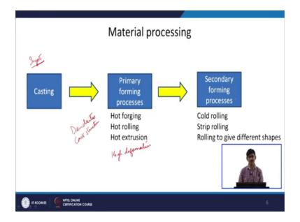
So, the first process by which we do is Casting. So, you basically melt the material and furnaces and then, you pour it into same ingots ok. So, we are not kind of concentrating here on different type of castings ok bulk material processing that you do casting in ingots ok.
