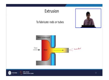
Extrusion is a another very important process to make rods or tube ok. So, if you put a mineral here this called a mandrel, you can get tube out of that.
