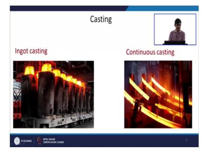
It is already lying on a rail and you can understand that the; what will be the dimension of this cast. So, basically from a big laden, where tons of molten metal molten metal is there it is poured into this kind of ingots where you get the shape of ingots maybe rectangular shape or round shape depending upon what processing you want to do later on ok.
