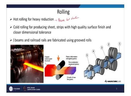
So, hot rolling is done for heavy reduction basically to break to break your cast structure ok. Once you do that in hot rolling the problem is because the material will be hot, there will be lot of oxidation takes place. So, you have scale on the surface.
