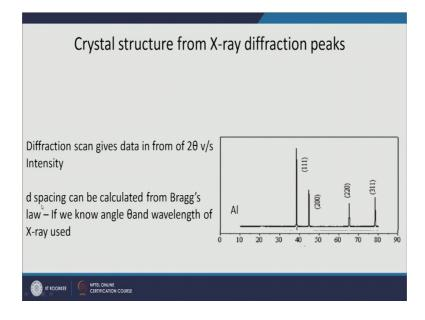
So, when you do a X-ray diffraction experiment you get what we call as this x axis is the two theta angles and the y axis is the intensity ok. So, it is intensity versus two theta angle.
