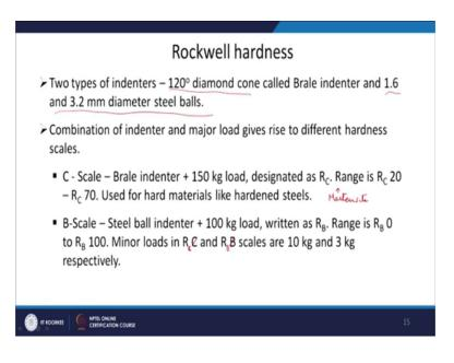
So, indenter is basically a diamond cone of 120 degree cone angle which is called a Brale indenter and 1.6 and 3.2 mm diameter steel balls are also used in case of Rockwell ha for finding out Rockwell hardness. So, either you will use this diamond cone or you can use these steel balls. Combination of indenter and measure ball the load give rise to different hardness scale ok.
