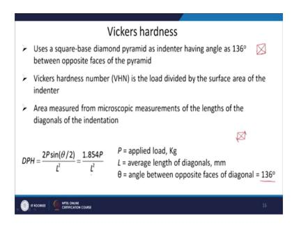
Which uses a square based Diamond pyramid. So, instead of cone, now you have a pyramid a square base pyramid.
