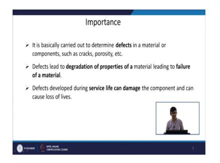
Importance: It is basically carried out to determine defects in a material or components, such as cracks, porosity etcetera. Why we want to know these defects because they will degrade your properties of a material and it may lead to failure of a material. So, if the defect or is of a critical size and the given stress condition in which your this component is going to be used, this crack can be can start propagating.
