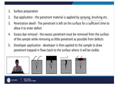
Then, we will apply the liquid or the dye on this surface, it can be applied by spraying or brushing whatever. Then this dye will penetrate ok. So, you have to give some time for it to penetrate these are liquid, it will penetrate through the crack.
