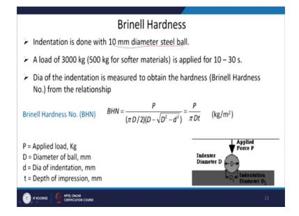
So, the first idea which was proposed to find out the hardness was at 10 millimetre diameter steel ball ok, kind you press in the material ok. So, the impression which it creates on the material, it will give you the indication of the hardness. So, if it is hard material and when I press this steel ball it will give you a smaller impression; if it is a soft material and I press the steel ball with the same load ok.
