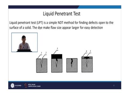
What we will do? I will show you the steps in the next slide ok. So, if this is the Liquid Penetrant Test is a simple NDT method for finding the defects open to the surface of a solid. The dye make flaw size appear larger for easy detection. So, basically liquid means we will be use dye, some colour and that we try to we try to enhance the size of the defect by this dyes, the liquid which we are going to use ok.
