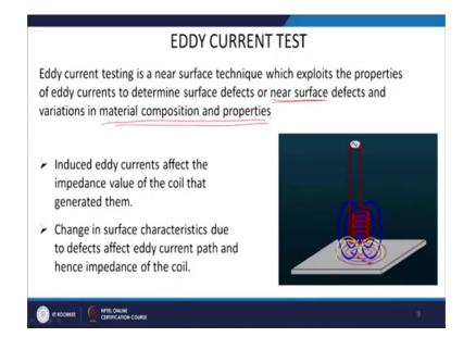
So, this is how the Eddy Current Test can be used to find out the sub defects near the surface ok. You do not have to be very open to the surface, it can be a subsurface defect also which can be easily find out with the Eddy current. And in fact, you can also find out if there is any material composition variation in the material ok. The other one is Ultrasonic Test ok. So, basically ultrasonic probe is there, which sends the ultrasonic wave in the material.
