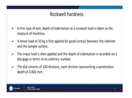
So, in this type of test depth of indentation at a constant load is taken as the measure of Hardness. In this case you are now applying a much smaller load than what we did in the Brinell hardness. So, 10 kg is applied for good contact between the indenter and the in the sample surface and then, you apply a major load.
