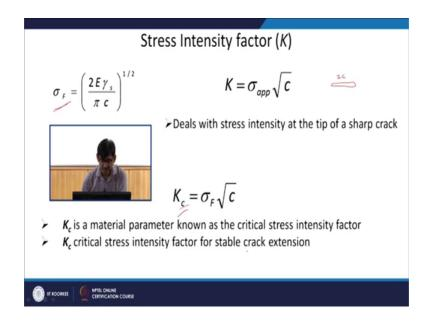
Then, we also said that in ductile material, because there will be some plastic deformation ahead of the crack. This actually stress will be more while we are talking about ductile material; that means you will need more stress to continue the crack or propagate the crack ok.
