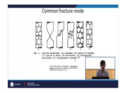
Just to recap here so, in this case the crack has going through the grain ok. So, and this is what we call as cleavage fracture through the through the crystallographic plane basically, the crack goes through the crystallographic planes.
