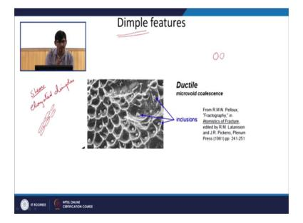
There is a precipitate sitting within the these dimples; that means, that the micro void might have nucleated there, then it is it was growing another micro void nucleated for this precipitate that is also growing and locally there is kind of a shear between the two of these holes. So, you have one micro void like this. Another micro void like this and when the material is whatever material is remaining between them ok, that is very thin small volume of material that will shear out.
