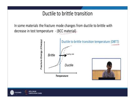
So, this is what we call as ductile to brittle transition. So, in some material the fracture mode changes from ductile to brittle with decrease in temperature and especially BCC materials are susceptible to this ok.
