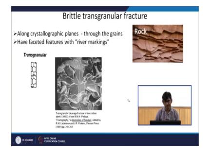
Brittle trans granular fracture ok; the crack is propagating along the crystallographic planes or through the grains and usually it gets you get a faceted feature with river markings faceted feature, because the crack is going along a certain plane.
