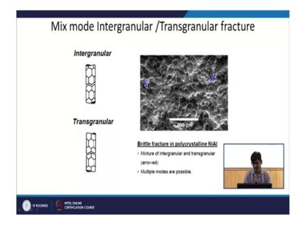
So, you can see these are all with faceted features ok, you can see a faceted feature here also ok. So, there can be some time mixing of two different fracture modes also because in practice things are not very simple ok. You have very complex stress system material is experiencing different stress state at different places.
