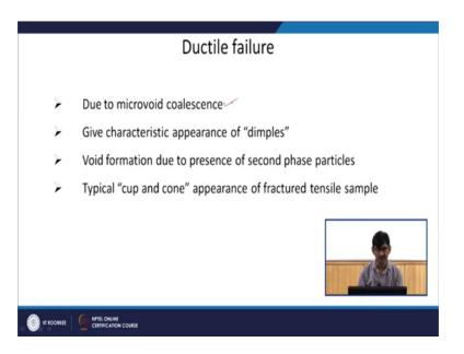
Due to micro void coalescence. So, we will see, what do we mean by that? Give characteristic appearance of dimples, actually this is what we call what features which we see on the; for ductile fracture ok. We say that these are dimples it looks like dimples wide formation due to presence of second phase particles and typical cup and cone appearance of fractured tensile sample.
