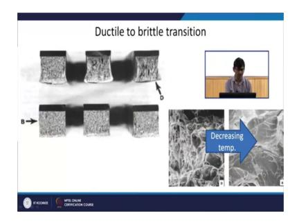
So, this is that ductile to brittle transition. So, the sample tested at different temperatures. So, at high temperature it behaves like a ductile material and at low temperature it will behave like a brittle material and the fracture morphology also changes, so as a function of decreasing temperature. So, here you can see that it is a ductile fibrous kind of appearance whereas, in this case you have faceted and river markings are there.
