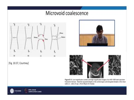
A necking starts at some point ok. Now, there will be some this kind of micro voids which will be forming on the inside the sample ok, why this micro void form ok. Suppose you have some inclusion in the material, let us say inclusion or precipitate or whatever and you are deforming. Now the mechanical properties of the precipitate will be different than the matrix ok. Usually precipitates are all very hard compared to the matrix.
