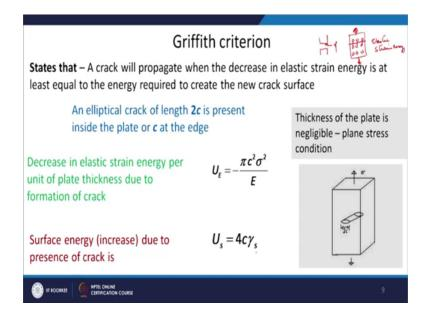
So, Griffith criteria propose that or states that that are crack will propagate when the decrease in elastic strain energy is at least equal to the energy required to create the new crack surfaces ok. So, what will happen when you have suppose material there are atoms here and you are applying a stress on the system ok.
