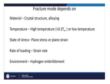
So, crystal structure or alloying already we have seen that different crystal structure and behave differently temperature as I told you that the temperature plays very important. So, in bcc material as a function of temperature it will either show as a brittle fracture as a brittle material or fracture as a ductile material ok. So, temperature plays very important role here state of stress whether it is a plane stress condition or plane strain condition rate of loading strain rate ok.
