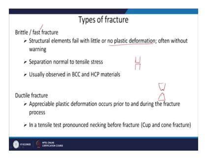
So, brittle fracture in this you do not have any plastic deformation or very small plastic deformation and that is why there is no warning ok. So, you will not know when you have reached the, the fracture stress of the material whereas, as you when you are plastic deformation it will take lot of time in getting deformed and then go into the fracture mode ok. And before that you will actually be able to see that something is deforming out of shape.
