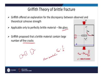
So the reason for bringing down this theoretical strength is that there are fine cracks present ok. So, first time it was proposed by Griffith ok, so and he proposed that for brittle materials because fracture process is very easy to understand in brittle materials because there is no plastic deformation; so only the separation between the two materials through breaking of the bonds without any plastic deformation.
