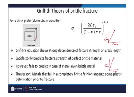
This slight change from the previous condition, so a 2 e gamma s by c. So, 2 e gamma s by 1 minus new pi c, so there is a additional contribution of poisons ratio here because we are considering the thick plate ok. So, thickness is more in this direction ok.
