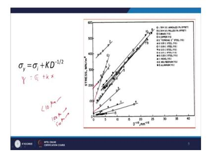
Large number of materials are written here 3 not 4 stainless steel brass copper some 0.05 carbon steel 0.09 carbon steel and so on, some nickel molybdenum and aluminum and
