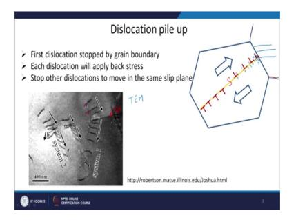
And the source is emitting the dislocations when you are applying a shear stress like this, and this dislocation will move and when they see a barrier grain boundary is a very strong barrier. The reason is that suppose my dislocation is moving on a crystallographic plane like this ok, in the next grain suppose is the next grain .
