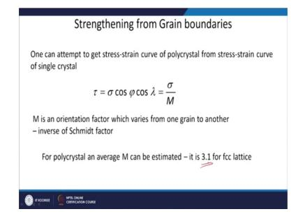
Ah you can give relationship, similar to what we saw in the single crystal that tau is equal to sigma cos phi cos lambda ok, and this cos phi cos lambda you can replace by sigma by m ok, where m we are saying is an orientation factor which varies fromone grain to another and this is a inverse of a schmidt factor ok. And for poly crystal and average m can be estimated it is around 3.1 for f c c lattice.
