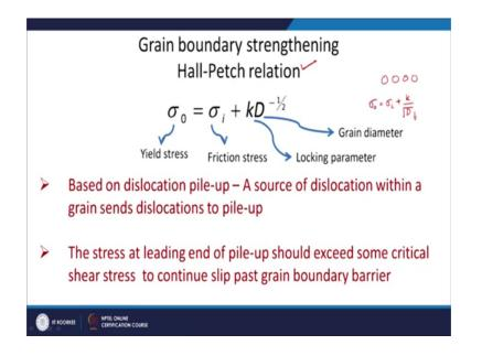
Or you can say sigma y also that is equal to yield stress depends on the sigma i friction stress, frictional stress is nothing, but for example, when I have an atomic arrangement and I have to move the dislocation ok. So, from for the movement of the dislocation i there is kind of a friction imposed by the lattice ok.
