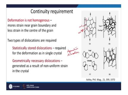
So if I allow these each of these grains to deform independently. So, there is no constraint what will happen that this will want to deform in whatever manner it will go it will go in this direction, the this one would like to go in this direction some some other gain will like to go in any direction.
