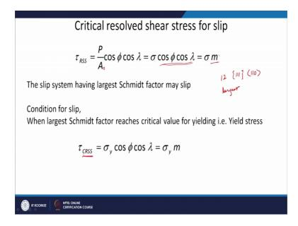
If this factor reaches the critical resolved shear stress, then the slip is going to take place.
