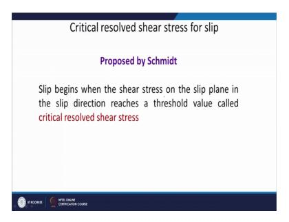
So, he said that when the a resolved stress in that particular plane and in that particular direction, when it reaches a critical value then the shear then the slip process will take
