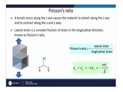
Now, after understanding the elastic deformation and Young's modulus, there is another very important parameter when you are doing deformation and the elastic limit is called Poisson's ratio ok.
