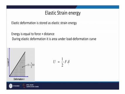
Now, there is another concept called elastic strain energy. As you see that when I am deforming it my potential energy is increasing; that means, I am storing the strain energy in the material, of course, elastic strain energy in this case because we are doing it under elastic limit. So, elastic deformation is stored as elastic strain energy in the material and how what do we mean by energy, energy is equal to force into distance.
