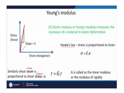
So, this is how elastic behaviour will look like in a typical stress strain curve ok. So, you have stress on the y axis and strain on the x axis.
