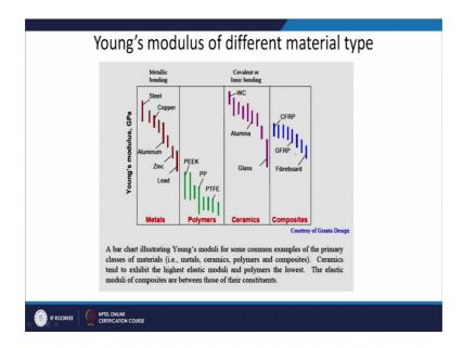
This is what is the driving force for elastic deformation. These are some values of Young's modulus of different material type ok. So, you can see that covalent or ionic bonds are a very strong bond. So, very high elastic modulus and this is for metallic bonds steel has very high long elastic modulus than copper aluminium zinc depending upon their bond strength ok. They will be grouped in different categories here some for polymers also are shown here polymer and composite.
