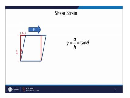
Similarly there can be shear strain which will be because of the force applied to the parallel to the area. So, suppose this is my initial object and I am applying a force here in
