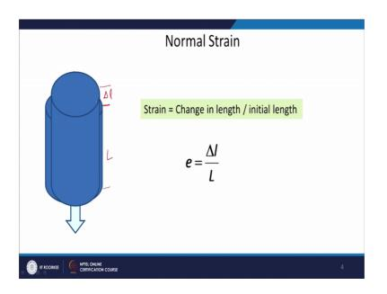
So, basically I when you apply a force like this ok, I am have changed the length. So, initial length let us say for my material was L and change in length is let us say given by delta l ok, then the strain will be change in length which is delta l divided by the initial length that will be equal to the normal strain again because I am measuring the strength on the area which is normal to the stress ok. So, I will call it as normal strain.
