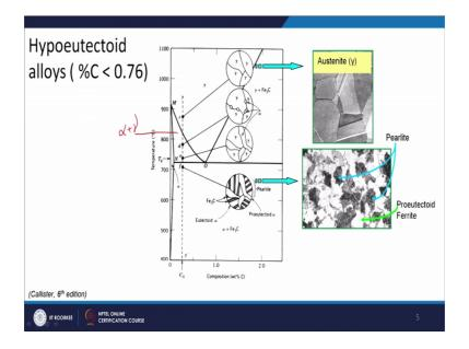
So, when you are a in austenite phase you will have a austenite microstructure which will look something like this ok, the austenite phase maybe that microstructure, that is transforming into at the eutectic point eutectoid point it is this asteroid is transforming into alpha plus Fe3C that is what we said and as he we discussed in eutectic system that when you have 2 phases coming from a single phase ok, the most appropriate is usually is that they form the 2 phases in close vicinity.
