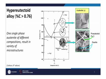
You see that some cementite which has started nucleating on the grain boundaries of austenite, the earlier it was ferrite which was nucleating here now it is cementite which is nucleating yet, because this region contains the equilibrium between austenite and cementite.
