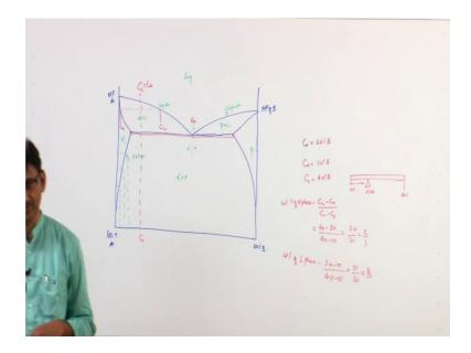
Overall C naught is equal to 20 percent B and from here we are saying that the C alpha has the composition 10 percent B and C liquid has composition 40 percent B. Now I want to find out the suppose these are in weight friction what will be the weight fraction of alpha phase, for example weight percentage of alpha phase.
